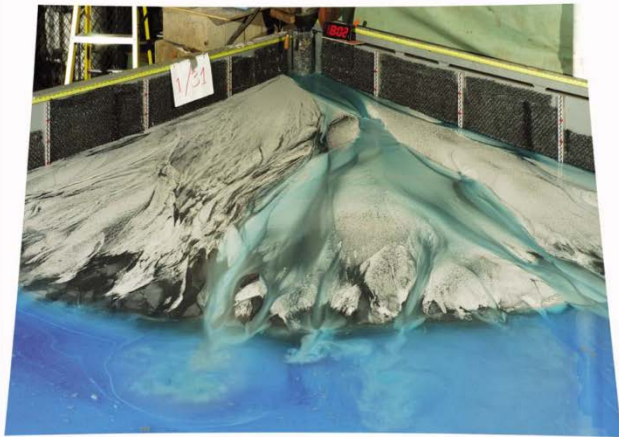
419 Figure 4. Example of an experiment using an analogue-landscape modelling approach (Sheets, 420 Hickson, and Paola 2002; Ganti et al. 2011). (a) Schematic of the experimental set up. (b) 421 Photography of the delta after 11 hours of experimental run time. From Ganti et al. (2011).
