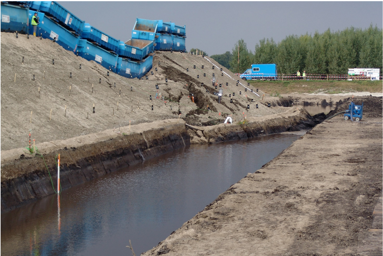
190 Figure 3. Example of a physical model of a river dike taking a 1:1 approach 191 ( http://www.dijkmonitoring.nl/en/projects/ ).
