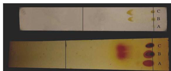
**Fig. 3** TLC analysis of the reaction mixture, shown in scheme 1, on a silicon diimide plate (top) and a silica gel plate (bottom), run using a (95:5) mixture of hexane:dichloromethane as eluent. A is a spot of the phenol starting material. Spot B is a combined spot of the reaction mixture and the phenol starting material. Spot C is the reaction mixture shown in scheme 1.
