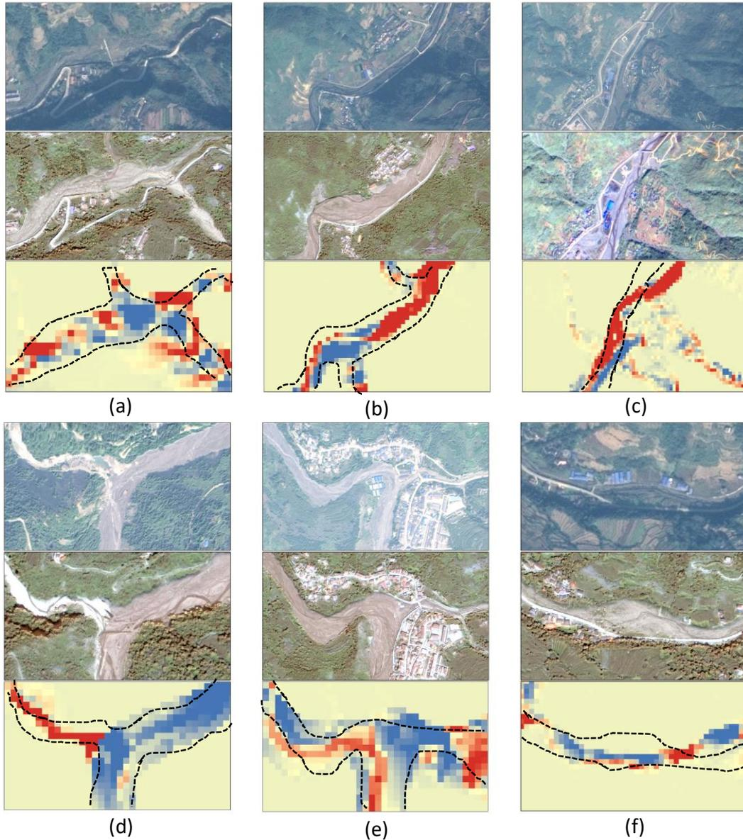
Note: Each site has 3 pictures. The picture of the first row shows image of 2012 before the flooding; second row shows image of 2013 after flooding; third row shows deposition (blue) and erosion (red) from the modeling results. The dash lines denote the observed impacted area along river channel from images and field reconnaissance.
