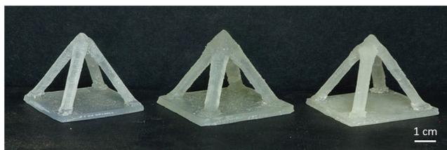
**Figure 4.** Photograph of 3D printed objects with various capsule loading values. From left to right the microcapsule loading increases from 0 to 5 and then 10 wt%.
