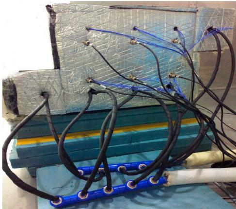
Figure 5. Image of the cold water supplying system.
