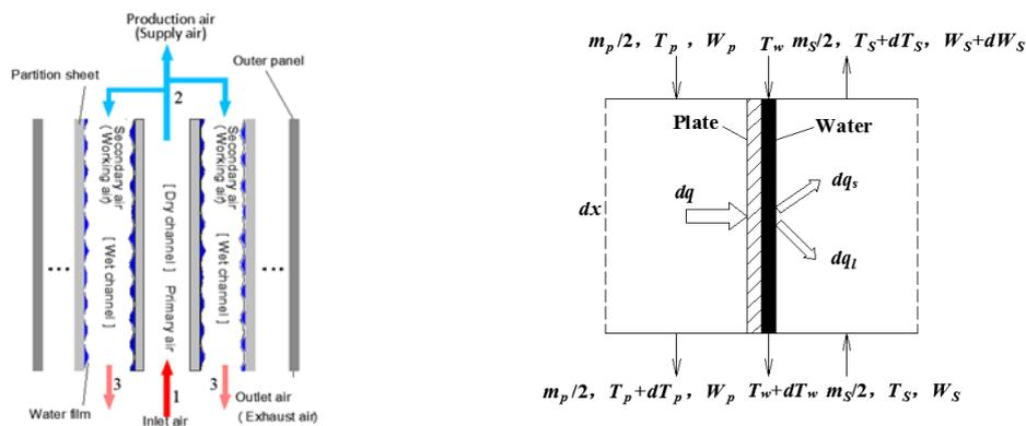
**Figure 1. Schematic of counter flow HMX Figure 2. cell control element applied for calculation**
