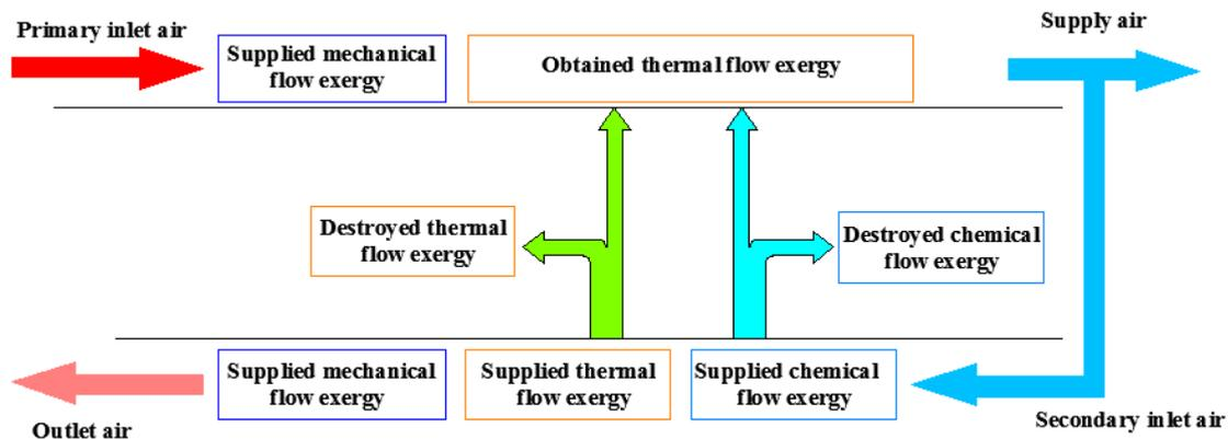
**Figure 3. The schematic diagram of exergy analysis**
