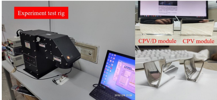
Fig. 2 The prototype of the CPV/D, CPV module and the indoor experiment test rig.
