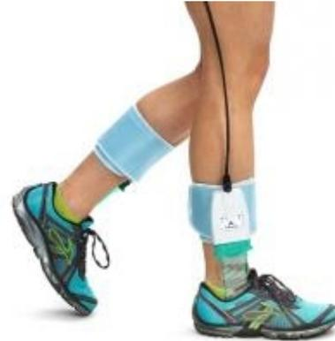
Fig. 1. The F-scan (Tekscan, Boston, USA). A Wireless telemetry system enabling freedom of movement, that uses soft, flexible sensors worn inside the shoe, connected to a data acquisition unit worn around the waist via data cables running up the legs. Examples of the data produced from this system can be seen in Figures 3 and 6.
