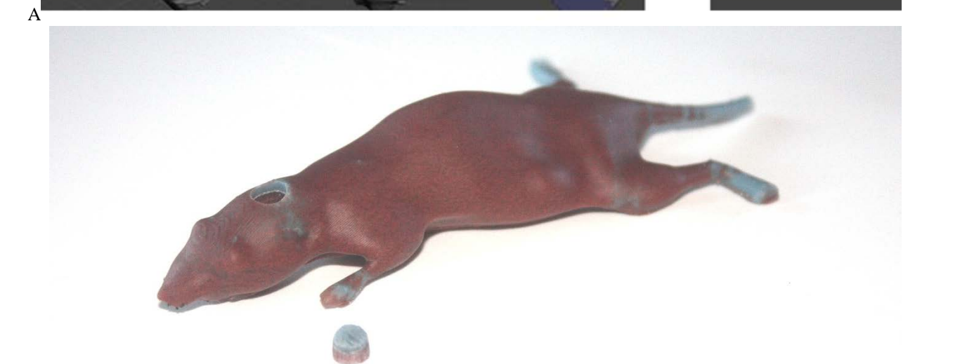
B Figure 4: Design of cavity and core insert for intracranial incorporation of alanine pellet into skull with skull 'cap', visualised in Meshmixer (A) and cored phantom with insert (B).
