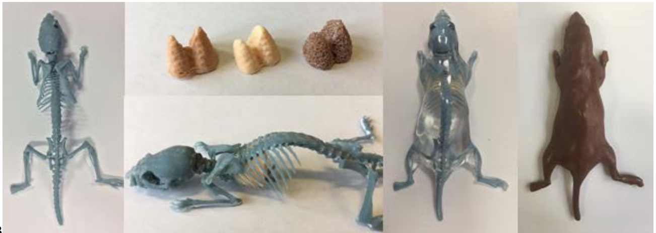
B Figure 3: Maximum intensity projections from CT scan of original animal and resulting segmentation illustrating bone, lung and soft tissue components separately and fused (Left to right respectively; A). Printed skeleton, milled lung inserts (LN330, LN450 and LN10), assembled skeleton/lung construct before whole body casting to create final phantom (B). Transparent Epoxy resin phantom allows internal structure to be seen for demonstration.
