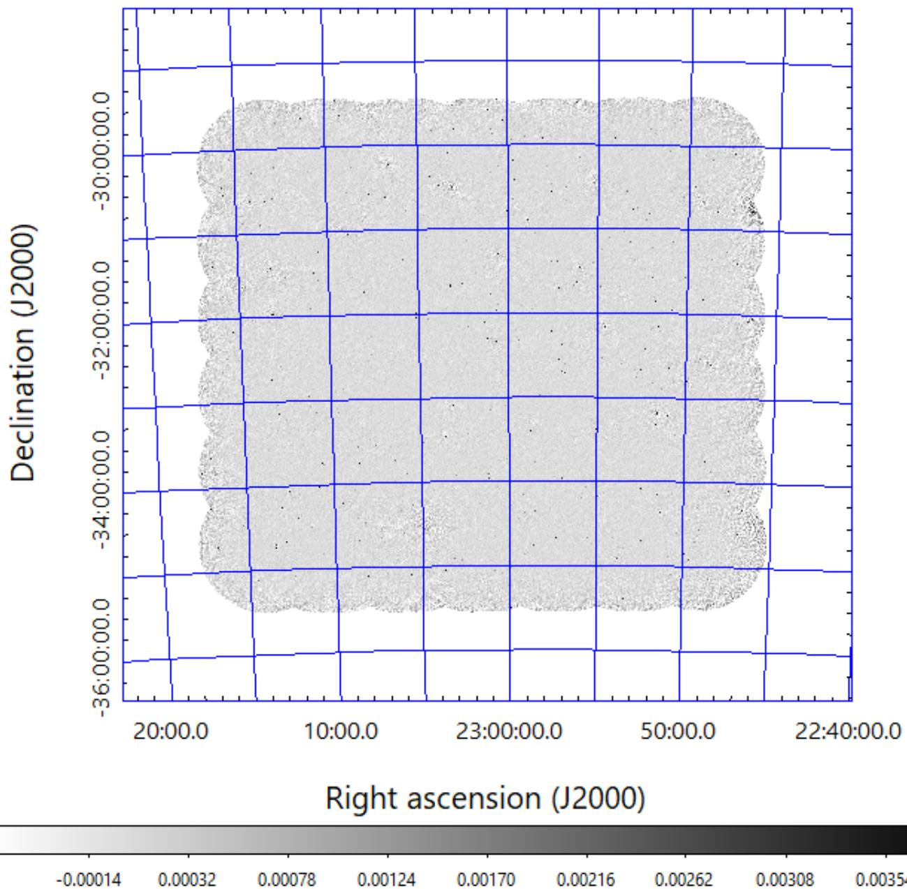
**Figure 3.** The 1320 MHz final processed radio image for the GAMA 23 region. This covers a sky area of  $\sim 6.6^\circ$  in R.A. by  $\sim 6.1^\circ$  in Dec. The greyscale bar at the bottom is in units of Jy/beam.
