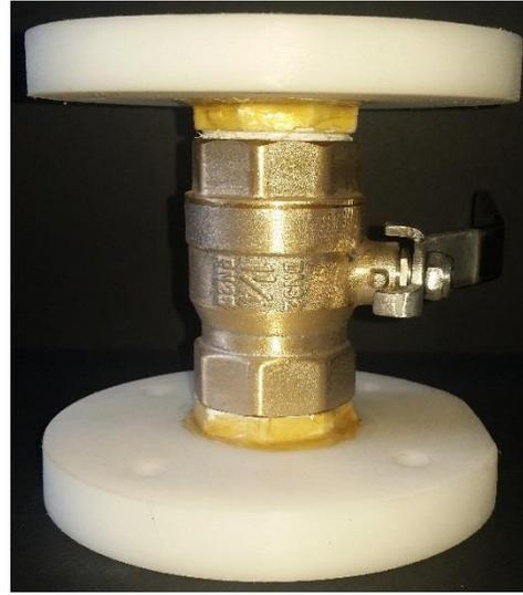
**Fig. 2.** Gate and ball valve used in the experiments
