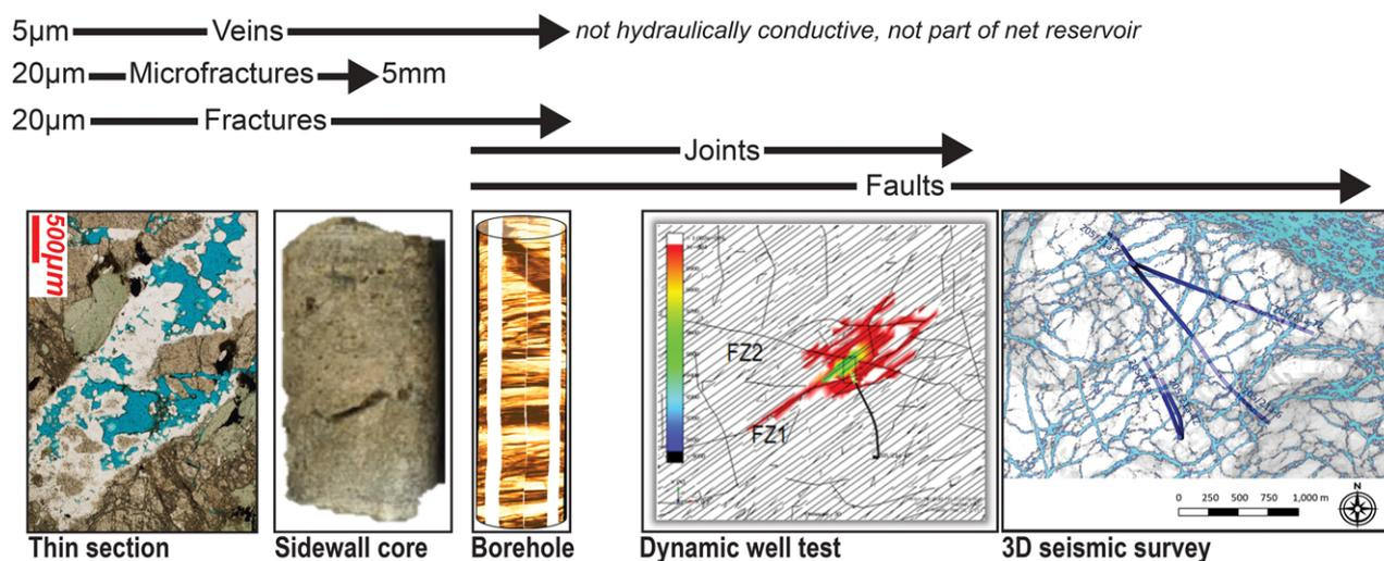
**Fig. 3.** The scales and classification scheme of fractures used for the Lancaster basement by [Belaidi \*et al.\* \(2016\)](#) and [Bonter \*et al.\* \(2018\)](#) and the range of data types used to image and understand these fractures.
