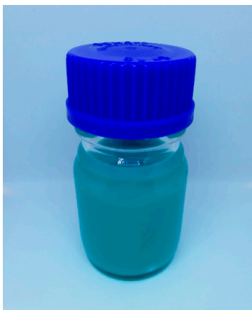
Figure A1. A mixture of 1.6\text{ g Cu(OAc)}_2\cdot\text{H}_2\text{O} and 1.5\text{ g OH-mBDC} in 100\text{ mL DMSO} after 2\text{ h} , showing a precipitation occurred in [\text{Cu}_{24}(\text{OH-mBDC})_{24}]_n stock solution.
