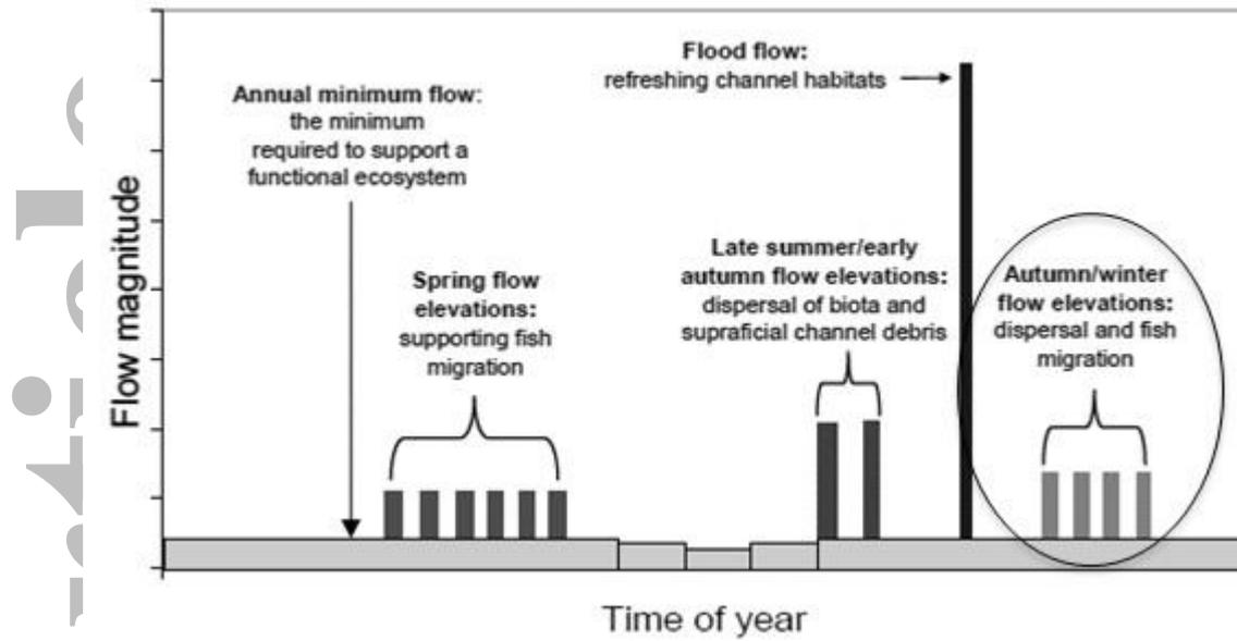
Figure 1. Schematic representation of a mitigation flow regime based on the recommended flow ‘building blocks’ (from UKTAG, 2013), including autumn/winter flow elevations for fish dispersal and migration (black circle).
