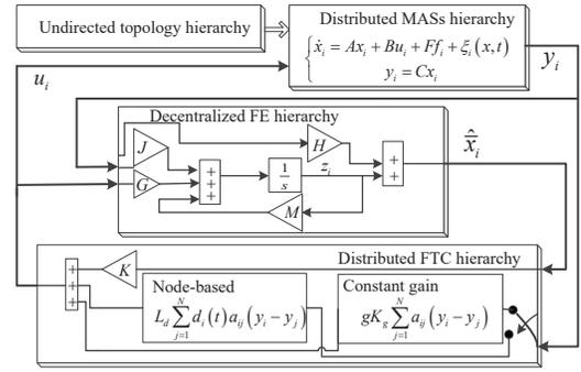
Fig. 2. The hierarchical structure-based FE and FTC algorithm.
