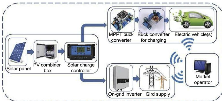
Fig. 2. S2V block diagram with smart grid concept.
