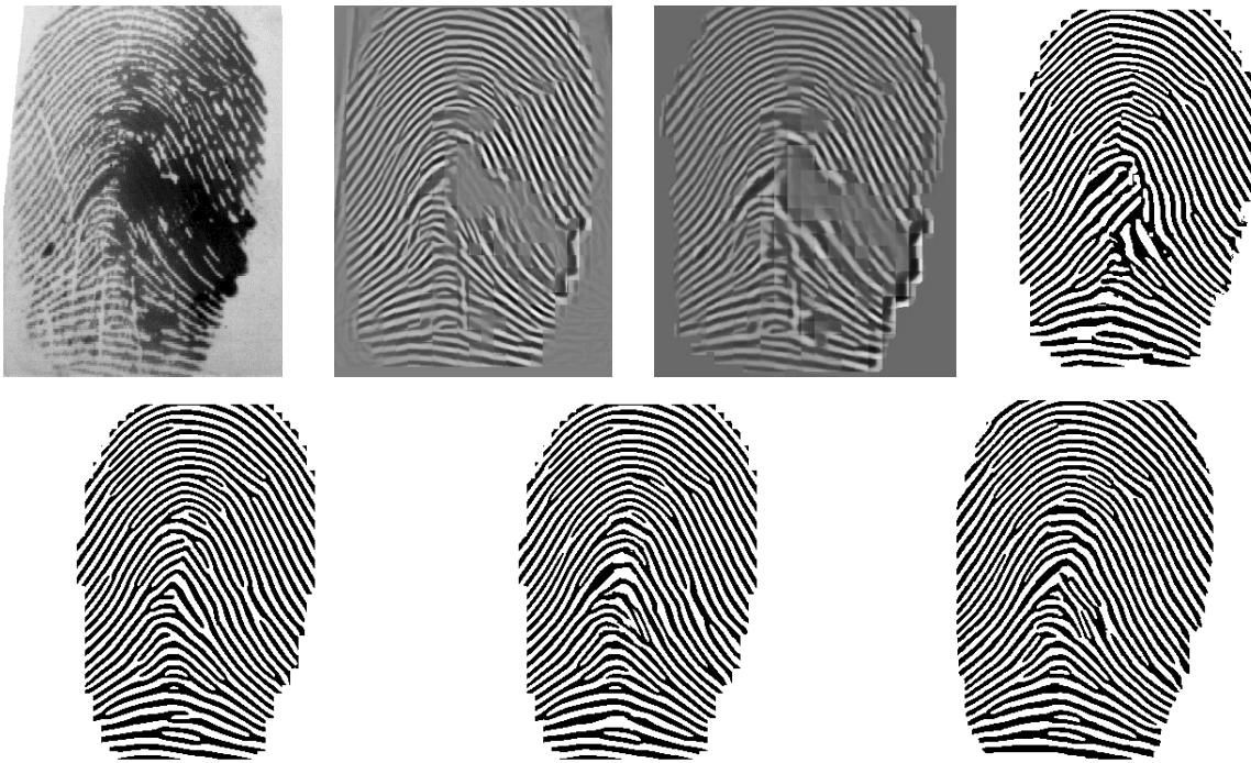
Fig.9. The fingerprints enhanced by various method, the original fingerprint image comes from FVC2004 DB2_4_8. The original fingerprint is shown in row 1 column 1. Correspondingly, the enhanced fingerprints by Gabor filtering method [6], STFT method [15], ABSF method [16], ACBF method [17], CDL method [31] and proposed method are shown from row 1 column 2 to row 2 column 3.
