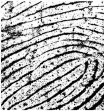
Figure 3. Chemical Imaging of a fingerprint: Time of Flight (TOF) SIMS image of potassium ( K^+ ) in a fingerprint deposited on brass, showing third level detail.
