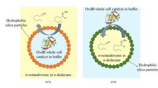
**Scheme 1.** Biocatalytic transformation of n-octanaloxime to n-octanenitrile carried out in Pickering emulsions (w/o and o/w) stabilised by silica particles of different hydrophobicity. Although the starting material and the final product are slightly soluble in the aqueous phase, this has not been included for simplicity.
