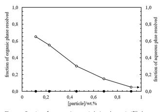
Figure 5. Fraction of aqueous (empty circles) and organic (filled circles) phase resolved from the o/w emulsions in Figure 4a prepared with different concentrations of 65% SiOH silica particles 1 month after preparation.
