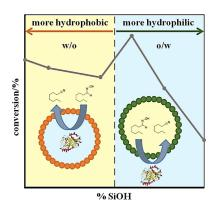
The dehydration of *n*-octanaloxime to *n*-octanenitrile catalysed by an aldoxime dehydratase (OxdB) overexpressed in *E. coli* is carried out in Pickering emulsions stabilised solely with silica particles of different hydrophobicity. The effect of particle wettability and particle concentration are evaluated with respect to the conversion of the reaction.
