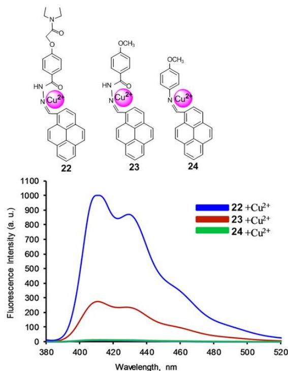
**Fig. 20.** Structure of chemosensors **22**, **23** and **24**. Fluorescence response of ligands upon addition of  $\text{Cu}^{2+}$  ions in  $\text{CH}_3\text{CN}/\text{CH}_2\text{Cl}_2$ . Reproduced from ref. 87 with permission from the Elsevier, copyright 2016.
