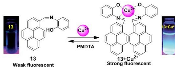
**Fig. 14.** Schematic presentation for detection of  $\text{Cu}^{2+}$  using receptors **13**. Photographs of **13** and **13**+ $\text{Cu}^{2+}$  visualized under UV-light irradiations. Reproduced from ref. 79, with permission from the Royal Society of Chemistry.
