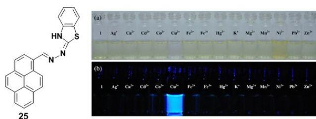
**Fig. 21.** Structures of probe **25** and Colour (a) and fluorescence (b) changes of chemosensor **25** (500 μM) after addition of various metal ions (500 μM). Reproduced from ref. 88 with permission from the Elsevier, copyright 2013.
