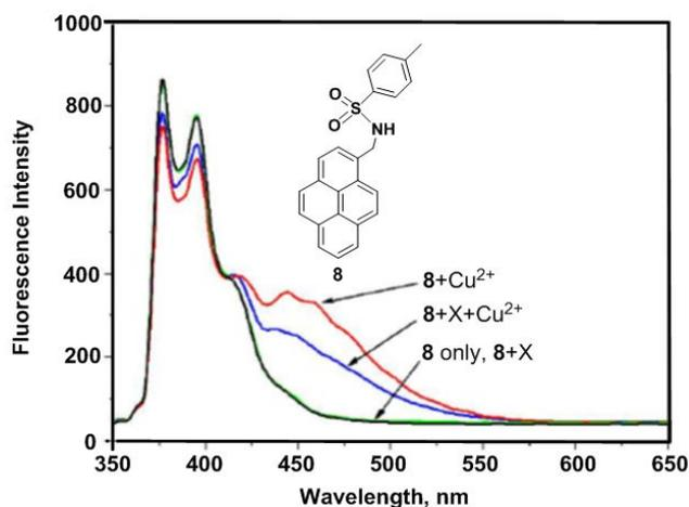
**Fig. 11.** The fluorescence spectra of **8** in the presence of  $\text{Cu}^{2+}$  and miscellaneous cations, **X** (10 equiv.). Reproduced from ref. 76 with permission from the American Chemical Society, copyright 2008.
