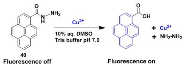
**Fig. 36.** The sensing mechanism of compound **40** with  $\text{Cu}^{2+}$  by catalytic hydrolysis process. Reproduced from ref. 107 with permission from the Elsevier, copyright 2017.
