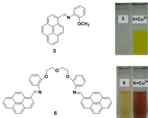
**Fig. 9.** Molecular structures of receptors **5** and **6**. Observed colour change **5** and **6** with  $\text{Cu}^{2+}$ . Reproduced from ref. 74 with permission from the American Chemical Society, copyright 2013.
