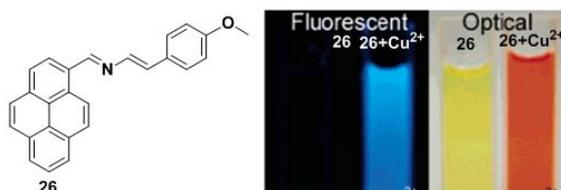
**Fig. 22.** Structure of chemosensor **26** and colour and fluorescence changes of **26** with  $\text{Cu}^{2+}$  in  $\text{CH}_3\text{CN}$ . Reproduced from ref. 89 with permission from the American Chemical Society, copyright 2006.
