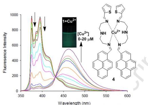
**Fig. 8.** Proposed binding mechanism of chemosensor **4** with fluorescence colour changes. Fluorescence Intensity changes of compound **4** ( $10 \mu\text{M}$ ) with different concentrations of  $\text{Cu}^{2+}$  in  $\text{Tris-HNO}_3$  buffer solution at  $\lambda_{\text{exc}} = 342$  nm. Reproduced from ref. 73 with permission from the Elsevier, copyright 2016.
