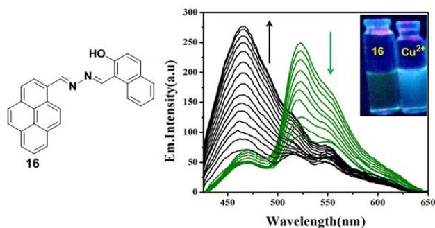
**Fig. 17.** Structure of compound **16** showing fluorescence emission spectra of **16** with the addition of  $\text{Cu}^{2+}$ . Inset: Visual fluorescence changes of **16** and upon addition of  $\text{Cu}^{2+}$  using a handheld UV lamp. Reproduced from ref. 82, with permission from the Royal Society of Chemistry.
