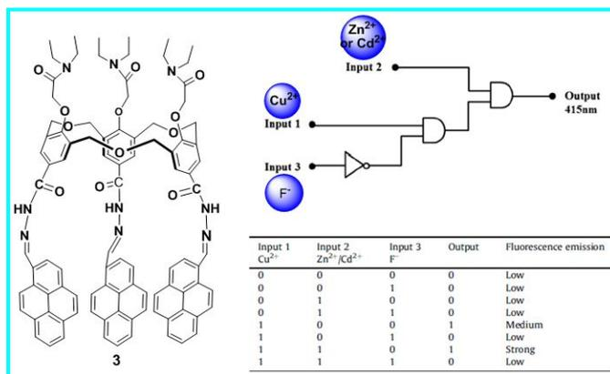
**Fig. 7.** The molecular structure of receptor **3** and the combinational logic gate for **3** with truth table using  $\text{Cu}^{2+}$ ,  $\text{Cd}^{2+}/\text{Zn}^{2+}$  and  $\text{F}^-$  as chemical inputs. Reproduced from ref. 72 with permission from the Elsevier, copyright 2015.
