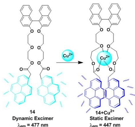
**Fig. 15.** Schematic representation of  $\text{Cu}^{2+}$  sensing by pyrene appended-binaphthyl-crown derivative compound, **14**. Reproduced from ref. 80 with permission from the Elsevier, copyright 2006.
