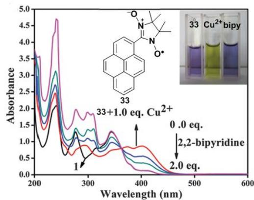
**Fig. 29.** The UV-vis absorption spectra of **33**+Cu<sup>2+</sup> and upon addition of 2, 2'-bipyridine in CH<sub>3</sub>CN. Inset: visual changes of the colour of compound **33**; compound **33**+Cu<sup>2+</sup>; compound **33**+Cu<sup>2+</sup>+2,2'-bipyridine (from left to right). Reproduced from ref. 96 with permission from the Centre National de la Recherche Scientifique (CNRS) and the Royal Society of Chemistry.
