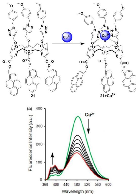
**Fig. 19.** (a) The structure of ratiometric sensor **21** and its binding mode with  $\text{Cu}^{2+}$ ; (b) showing fluorescence for the  $\text{Cu}^{2+}$  ion in  $\text{CH}_3\text{CN}$ . Reproduced from ref. 84 with permission from the Taylor & Francis, copyright 2015.
