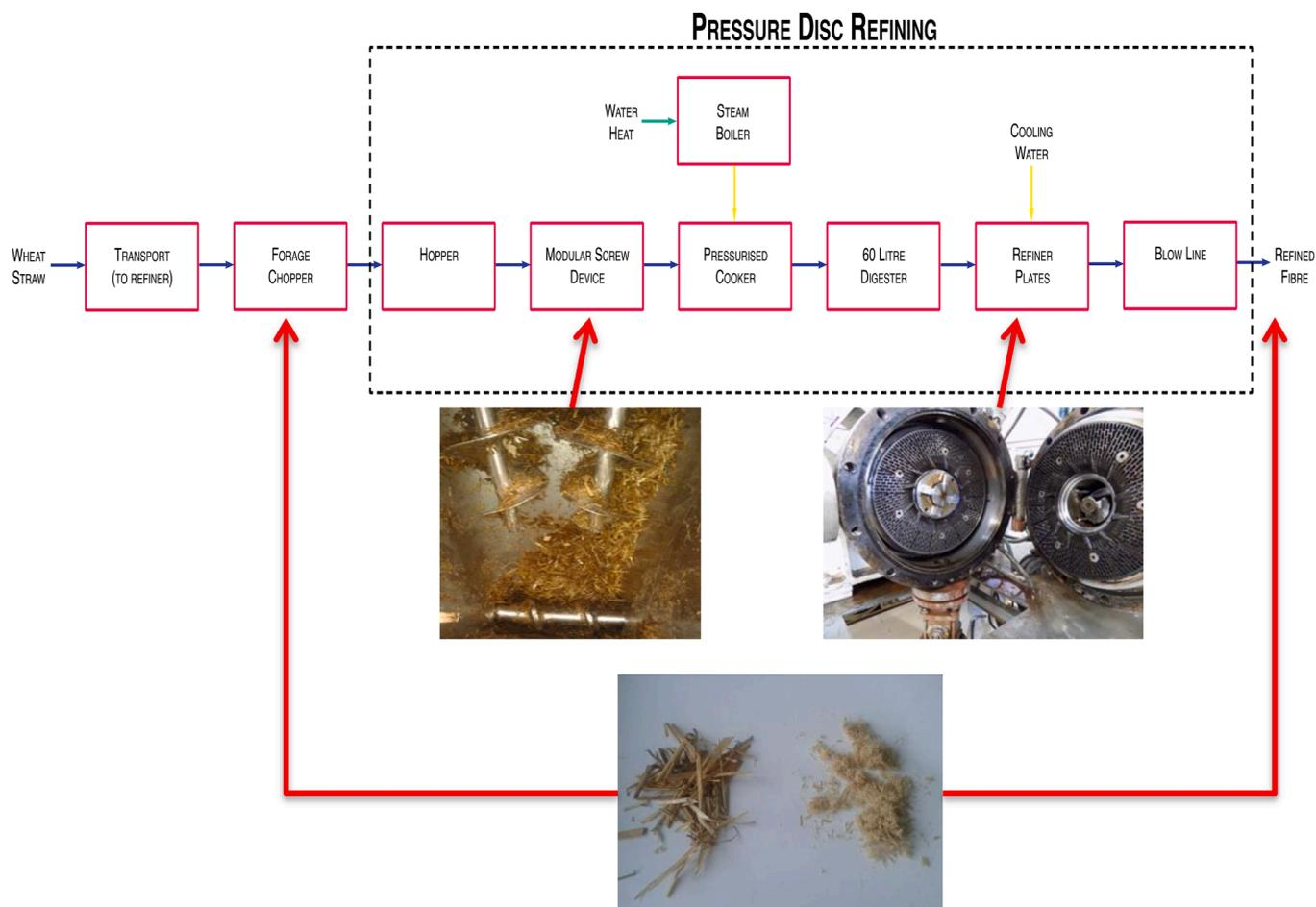
**Fig. 1.** Thermo-mechanical pre-treatment process used for the production of refined wheat straw fibre (top), with the modular screw device (MSD) and refiner plates showing the configuration of bars and grooves illustrated (middle). The difference in particle size between forage chopped wheat straw fibre and pressure-disc refined material is depicted (bottom).
