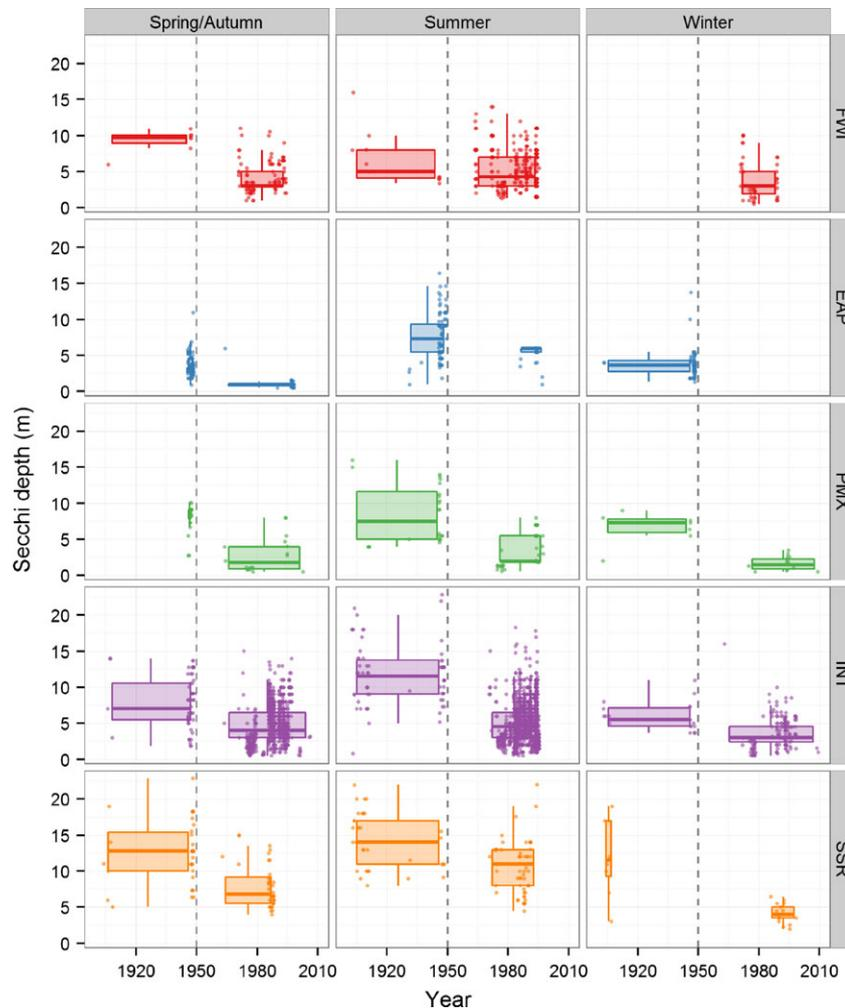
**Fig. 2** Observations of Secchi depth (m) for each hydrodynamic region and season. Points indicate individual observations of Secchi depth. Box plots show the median and the inter-quartile range of observations of Secchi depth pre- and post-1950. Abbreviations for hydrodynamic regions as in Fig. 1.
