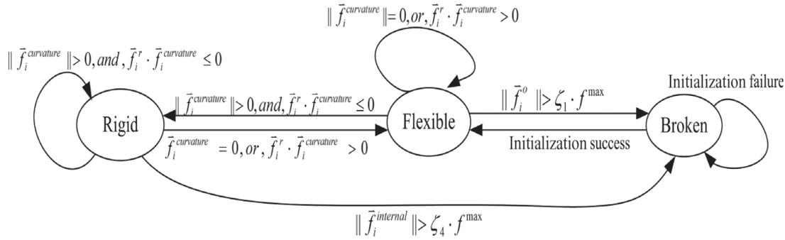
Fig. 2. State machine for state transition.
