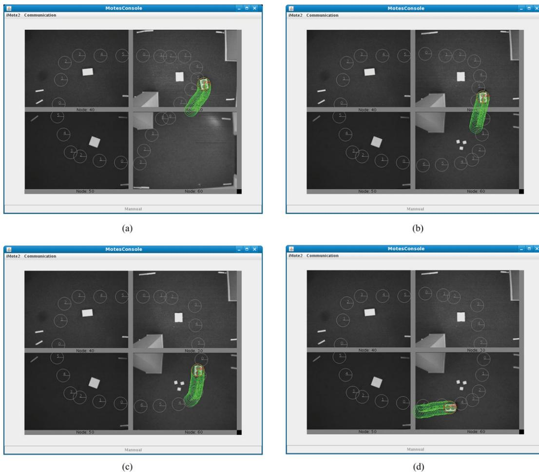
Fig. 11. (Colour online) The real-time experiments of robot control by a visual sensor network. (a) Snake without obstacles. (b) Obstacles appear. (c) Passing obstacle area. (d) Passed obstacle area.
