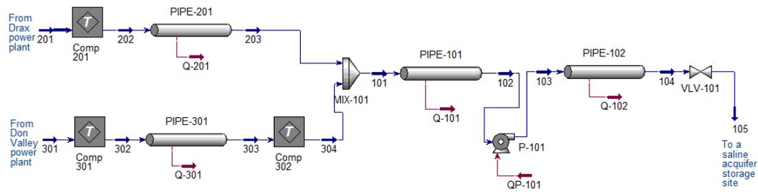
Figure 2. The flowsheet of pipeline network in Aspen HYSYS®
