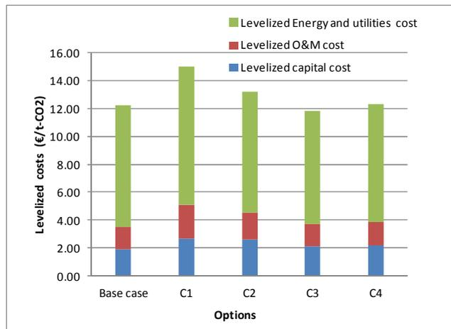
Figure 4. Comparison of levelized costs of different compression options
