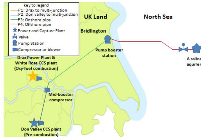
Figure 1. The pipeline sketch for the Humber case study
