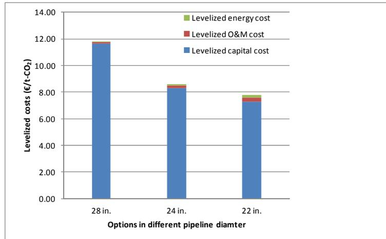
Figure 6. Levelized cost comparison for different diameters of the pipelines
