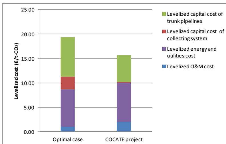
Figure 9. Comparison of levelized cost of the optimal case and COCATE project
