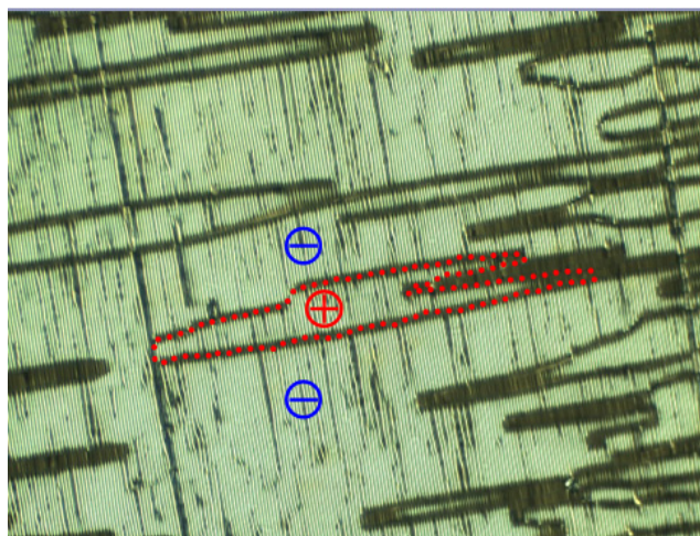
Figure 4. A 2 \mu\text{m} commercial (ECH ® , Japan) planar-aligned cell in the N_X phase [16]. Stripes observed are parallel to the rubbing direction. Discontinuities in the stripe pattern indicate the domain boundaries of opposite chirality. Identification of the chirality became possible via application of an electric field. The area marked by red dots corresponds to the domain of a single chirality, for example.
