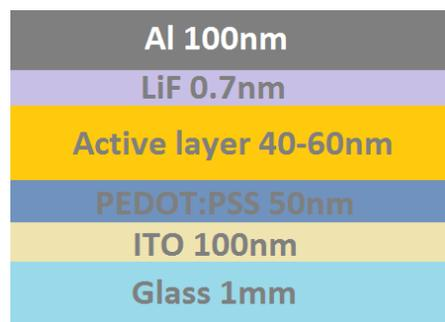
**Figure 4** PLED device stack, ITO: Indium-Tin Oxide.
