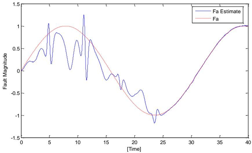
Figure 4: Fault signal  $f_a$  and fault estimate  $\hat{f}_a$  with AFTC activated at 20s
