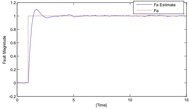
Figure 2: Fault signal  $f_a$  and its estimate  $\hat{f}_a$  with AFTC activated
