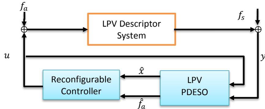
Figure 1: The structure of AFTC for LPV descriptor systems with PDES0
