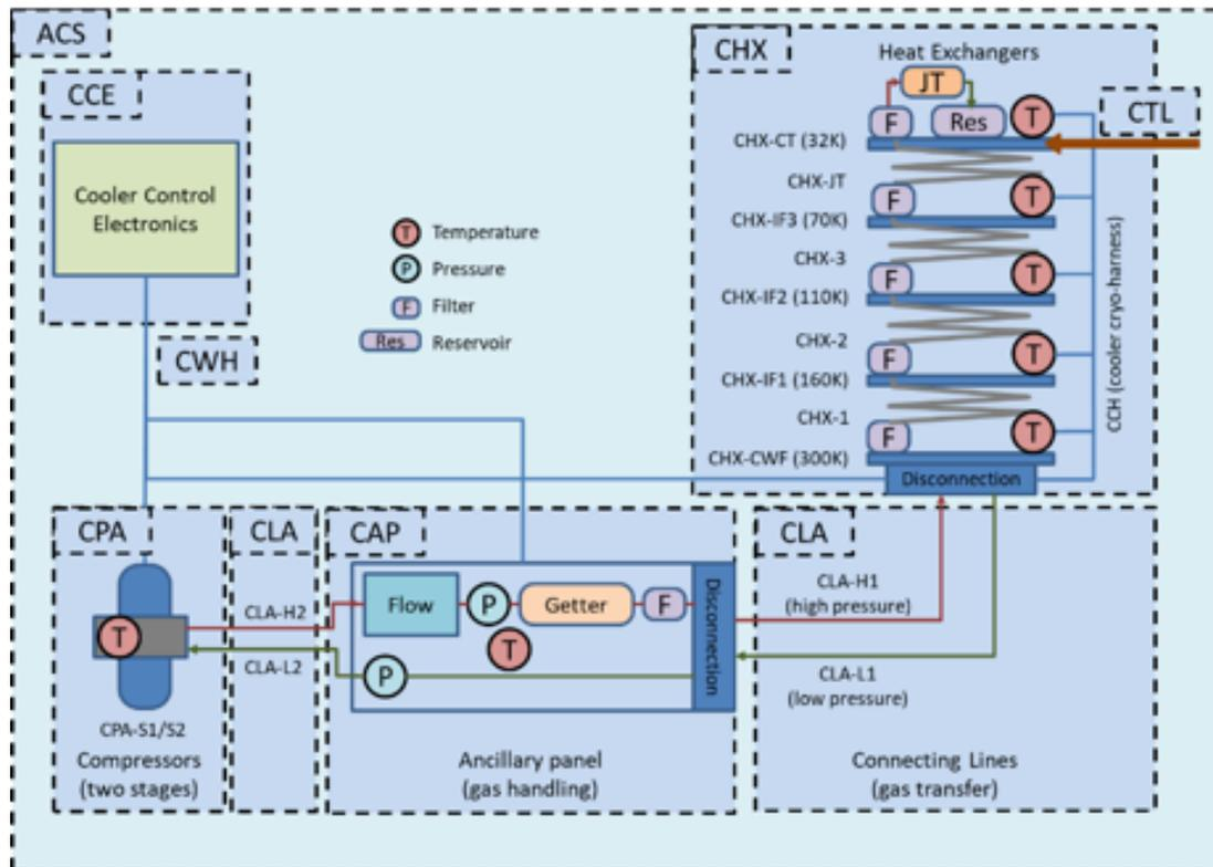
Figure 4-20: JT Cooler Schematic
