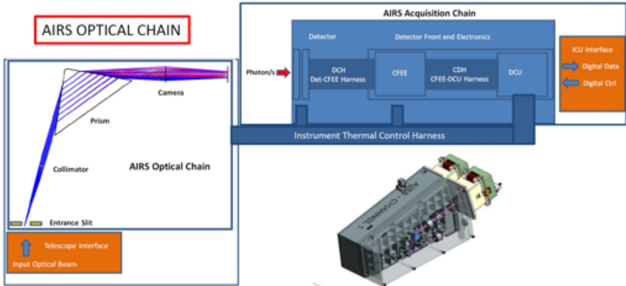
Figure 4-5: Architectural block diagram of the Ariel Infra-Red Spectrometer.
