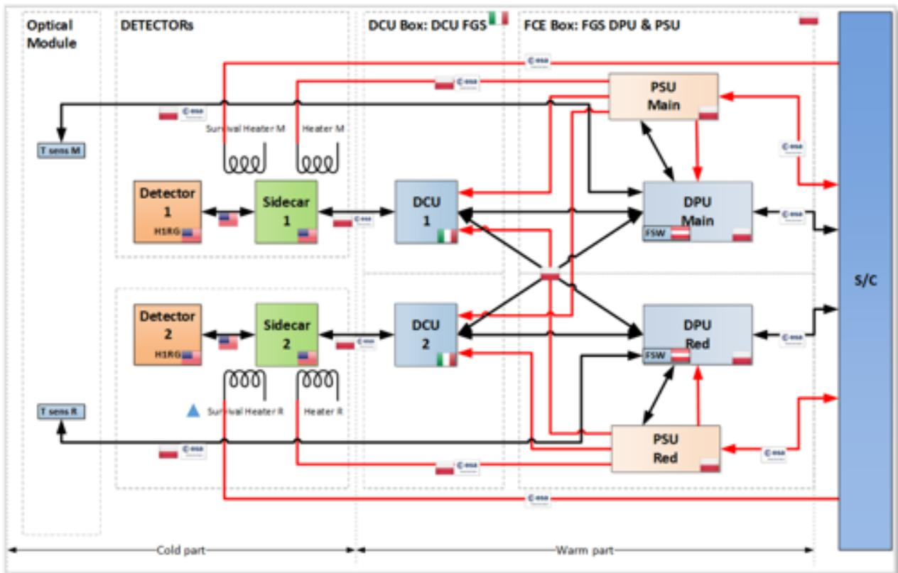
Figure 4-14: Scheme of the FGS control unit.
