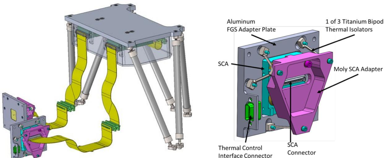
Figure 4-13: Conceptual design of the FGS detector system. Right – FPE (housing cFEE SIDECAR ASICs operating at  $\sim 130 \text{ K}$ , with cryo-flex harnesses running to detector modules. Right – Focal Plane Module (FPM) design
