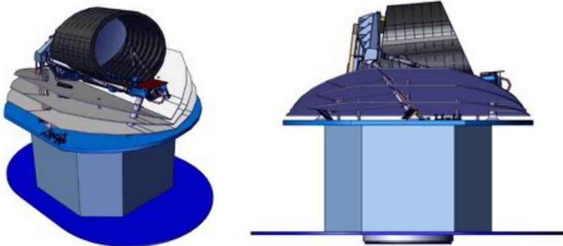
Figure 5-4: Illustrative representation of the Ariel S/C from two angles, composed of the Consortium provided PLM, and a generic dummy SVM. An upwards tilt (5°) can be seen on the right picture between the telescope pointing axis and the SVM “horizontal” XY plane. This means the accessible sky described in Figure 3-19 is a 50° wide annulus region near orthogonal to the ecliptic plane (-20° / + 30°)
