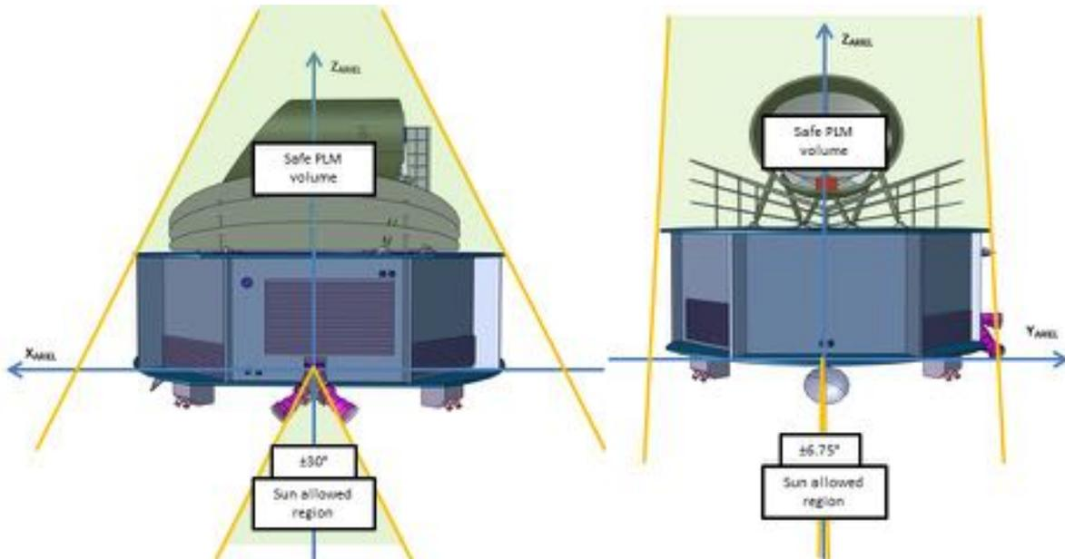
Figure 5-1: Ariel nominal cut angles and PLM shading (illustrative, not to scale). Left:  $\pm 30^\circ$  around Y. Right:  $\pm 6.75^\circ$  around X. In addition to the  $360^\circ$  slew capability around Z, this provides access to over 40% of the sky at any given time (requirement  $\geq 30\%$ ). Note that these cut angles include margin to accommodate for FDIR aspects. The resulting angular range that can be used for science observations is therefore a bit smaller.
