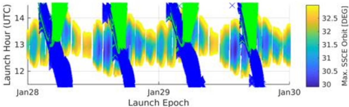
Figure 5-2: Example launch window for a direct transfer to L2 provided by ESOC (to be confirmed by Arianespace). Similar results are valid for any launch year. The colour scale indicates the resulting Sun-S/C-Earth (SSCE) angle in L2 as a function of the launch time. Launches resulting in eclipses during the transfer to L2 and during the nominal operations phase are crossed-out.
