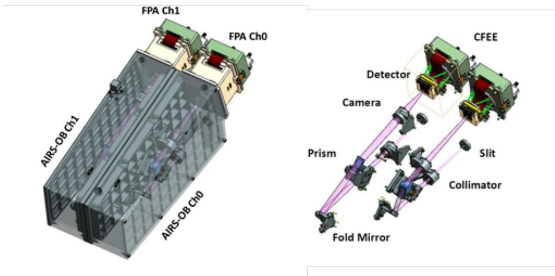
Figure 4-7: Implementation of AIRS optical design within the allocated volume. The size of the AIRS OB volume is  $482 \times 206 \times 184$  mm; the optical interface is at the slits which are 40 mm above the mounting plane and separated by  $\sim 108$  mm for the two channels.
