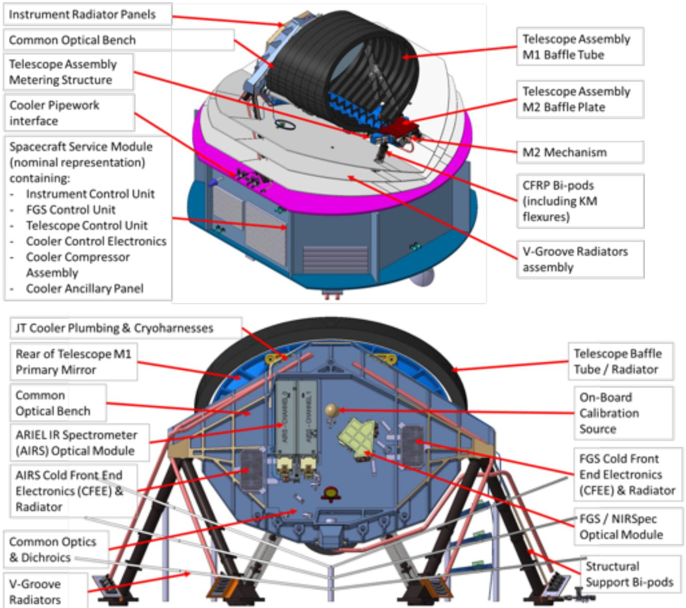
Figure 4-1: Ariel PLM overall mechanical configuration and layout.
