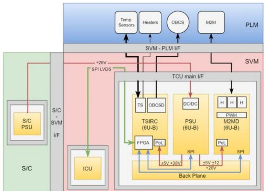
Figure 4-22: TCU block diagram and electrical I/F
