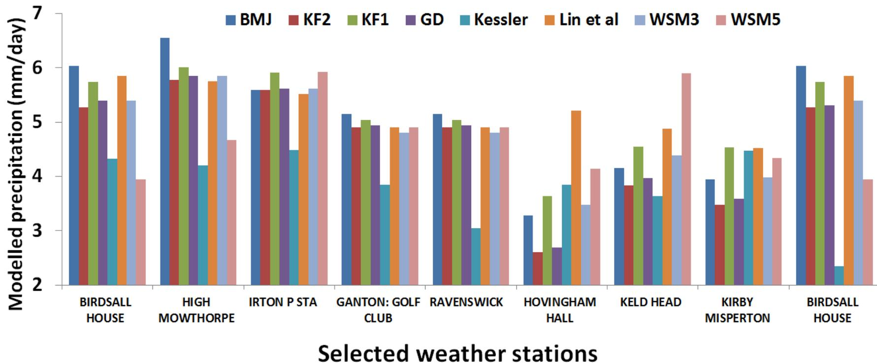
**Figure 6: WRF simulated precipitation under different CPSs /MPSs and observed catchment precipitations during ‘York Flood -1999’ corresponding to different weather stations [daily average of 1<sup>st</sup> March- 14<sup>th</sup> March 1999]**
