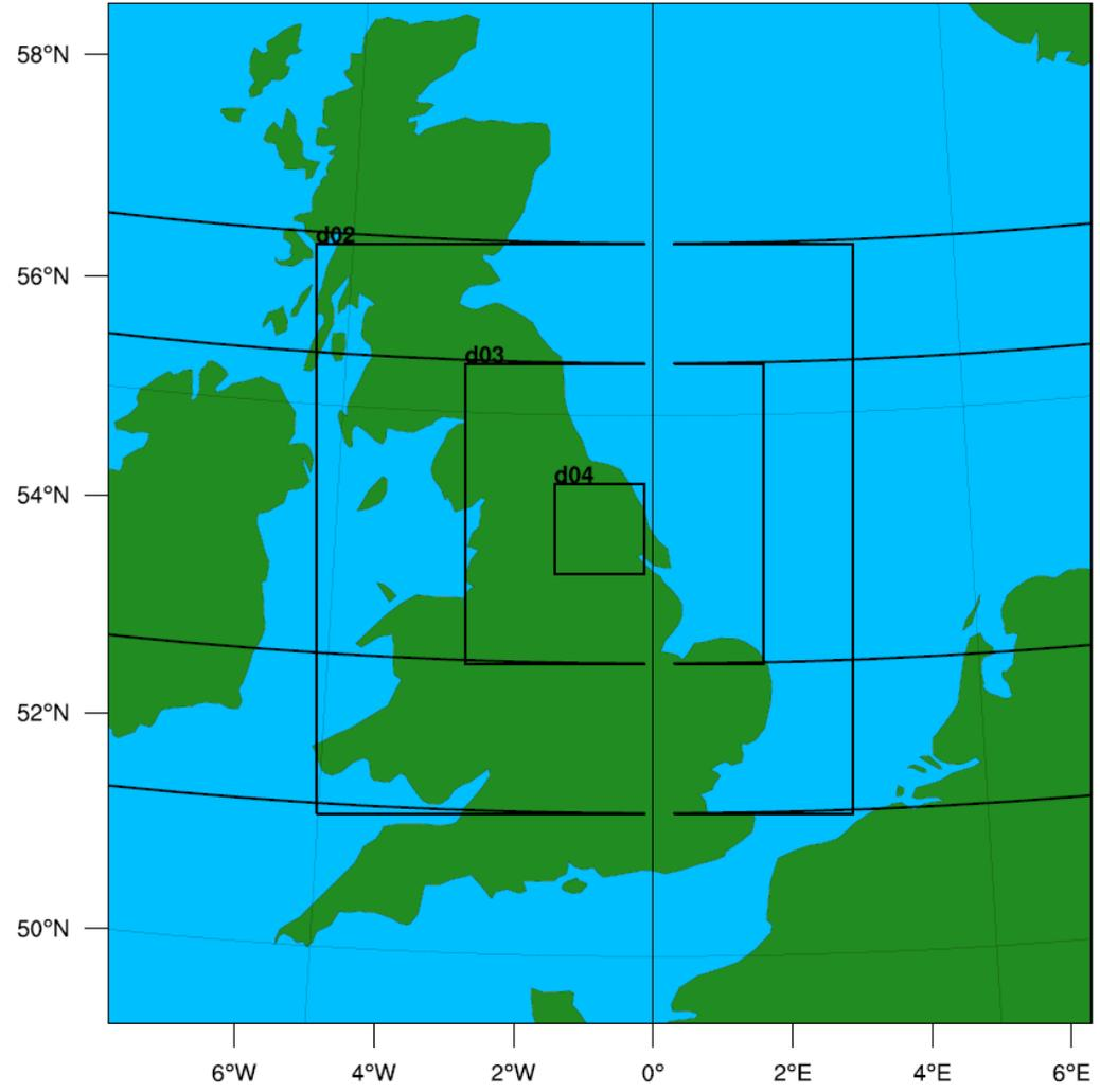
Figure 1 Dimensions of the nested domains for different model settings which are centred over the River Derwent catchment, Yorkshire-Humberside. d01, d02, d03 and d04 refer to the four domains (refer table 4 for details)
