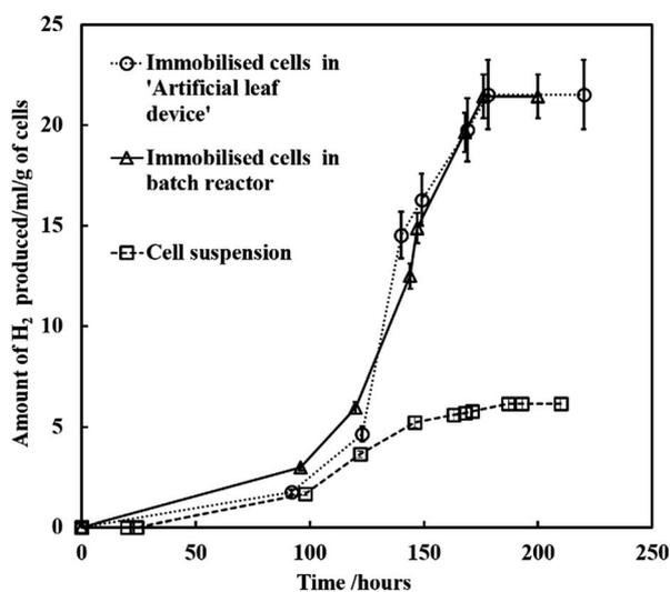
Fig. 9 The volume of the produced  $H_2$  gas (in mL) as a function of the incubation time per gram of suspended and immobilised *C. reinhardtii* cells in a 1 litre batch photobioreactor (dashed line and solid line) and the artificial leaf device (dotted line) in anaerobic condition suspended in TAP-P-S media in a system pre-flushed with argon. The three systems were illuminated with the same light source and media conditions.
