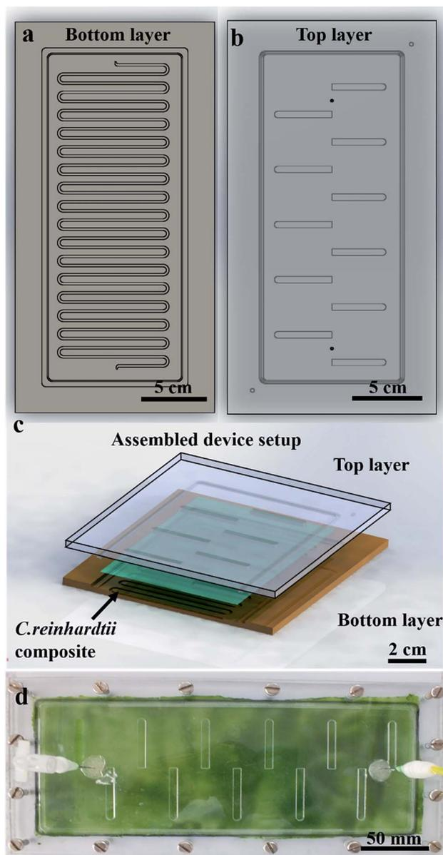
Fig. 4 Schematics of the components of the artificial leaf device (a) bottom layer, (b) top layer, (c) sandwiched *C. reinhardtii*-fabric composite between the top and bottom layer and (d) the photograph of *C. reinhardtii*-alginate fabric composite inside the assembled device.
