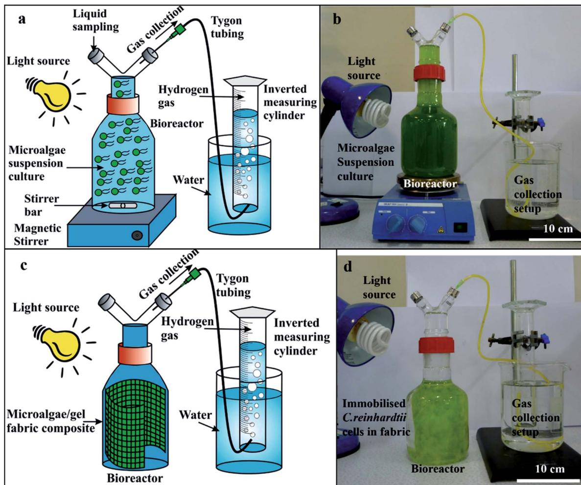
Fig. 3 (a) Schematics and (b) optical photograph of the batch photobioreactor for hydrogen production from *C. reinhardtii* cc-124 strain with an inverted graduated cylinder filled with water in order to measure the volume of hydrogen gas produced. (c) Schematics and (d) photograph of fabric-hydrogel-immobilised *C. reinhardtii* cells suspended in TAP-P-S medium in a batch reactor for bio-hydrogen production. Note that here the *C. reinhardtii* cells are not freely suspended in the batch medium.
