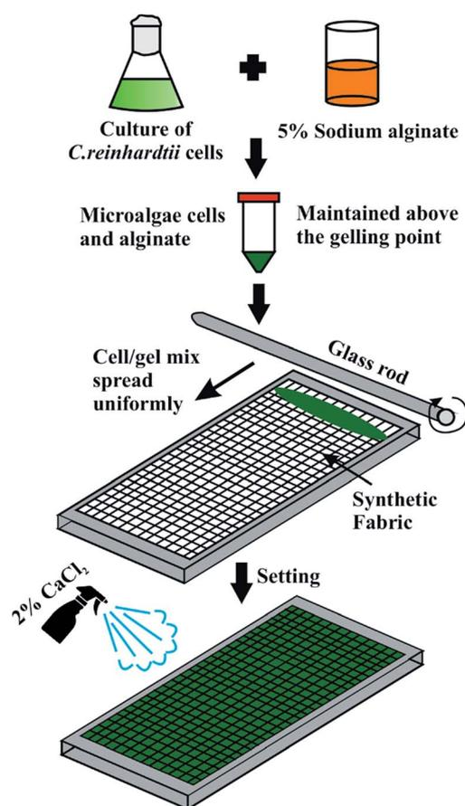
Fig. 2 Schematic of the microalgae immobilisation process. The *C. reinhardtii* cells were grown in suspension culture in aerobic condition and harvested by centrifugation. They were homogenised together with sodium alginate at 5% (w/v) concentration, poured over the synthetic fabric on a glass plate and spread uniformly over the fabric using a sterile glass rod. The alginate films were polymerised by spraying 2% CaCl<sub>2</sub> (w/v) solution.
