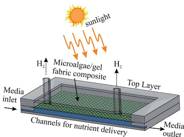
Fig. 1 Conceptual design of the artificial leaf device showing the vascular networks for nutrient delivery to the cells at the bottom and hydrogen extraction from above the *C. reinhardtii*-fabric composite.
