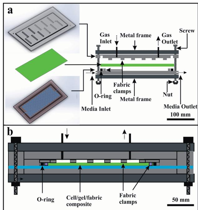
Fig. 5 (a) Expanded view of the 'artificial leaf device' showing the different parts of the assembly: the top layer, *C. reinhardtii* cc-124 composite and the bottom layer. (b) Schematics of the cross-section of the assembled device. The thickness of the compartments and the biocomposite layer is not in scale on this diagram.
