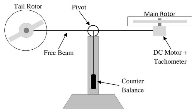
Fig. 1: TRMS model supplied by Feedback Instruments Ltd.
