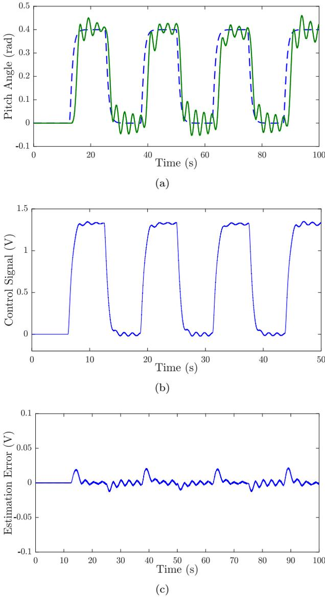
**Fig. 2:** The input and output of the TRMS system (a), control signal (b) and Kalman filter tracking (c) using the LQG controller with  $\mathbf{Q} = \text{diag}_{4 \times 4}(60, 60, 60, 60)$  matrix with diagonal elements equal 60,  $\mathbf{R}$  is  $1 \times 1$  matrix having a value = 10,  $\mathbf{W}$  is  $1 \times 1$  matrix = 1000, and  $\mathbf{V}$  is  $1 \times 1$  matrix = 1.
