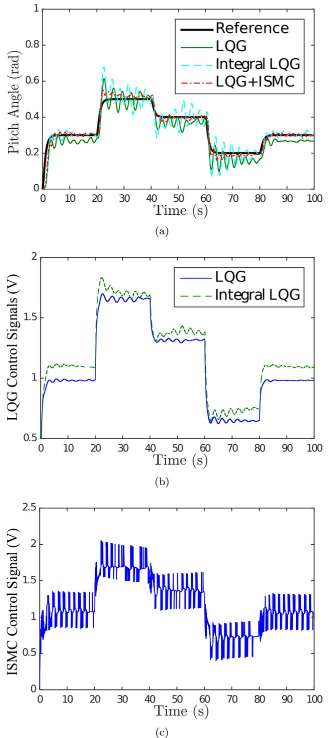
**Fig. 6:** ISMC-LQG experimental results for a multi-step input (a) and the corresponding control inputs for LQG and Integral-LQG (b) and for the LQG+ISMC (c). The main control parameters were chosen as  $\alpha = 0.3$ ,  $\delta = 100$ ,  $K_i = 1$ ,  $K_r = 1500$ ,  $\mathbf{Q} = 150$ ,  $\mathbf{R} = 100$ ,  $\mathbf{V} = 1$ , and  $\mathbf{W} = 1000$ .
