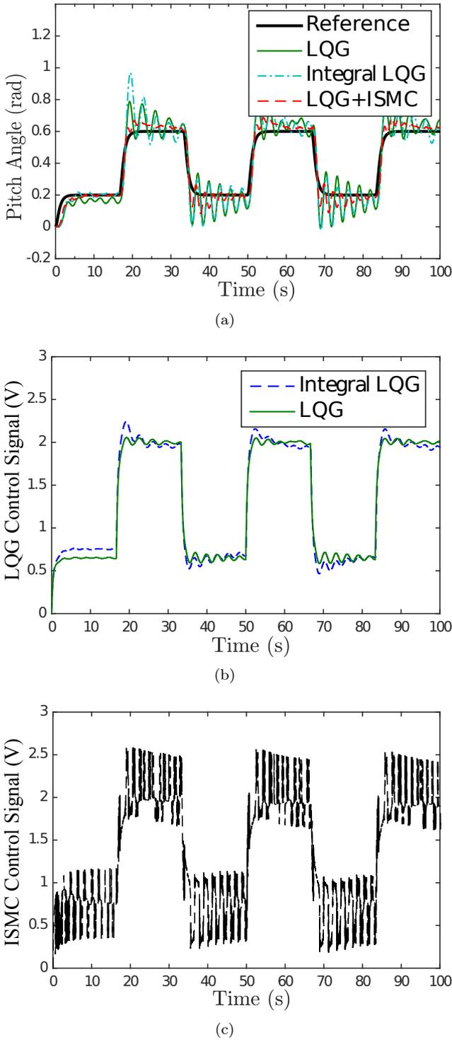
**Fig. 5:** Experimental results for a square wave demand using LQG, LQG with an integral action and ISMC (a) along with the corresponding control signals (b) and (c) with  $f = 0.03$  Hz,  $\alpha = 0.3$ ,  $K_i = 1$ ,  $K_r = 1500$ ,  $\mathbf{Q} = 50$ ,  $\mathbf{R} = 100$ ,  $\mathbf{V} = 1$ , and  $\mathbf{W} = 1000$ .
