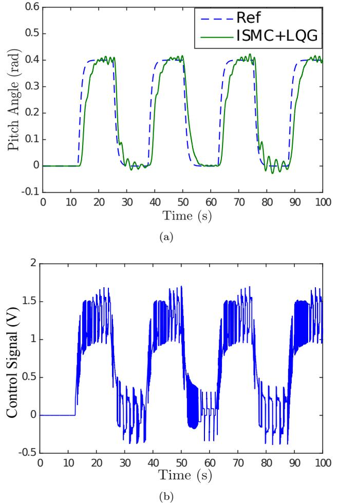
**Fig. 4:** ISMC-LQG experimental results for a square wave input with an amplitude of 0.4 radians and a frequency of 0.04 Hz (a) and the control signal (b). The main control parameters were chosen as  $\alpha = 0.3$ ,  $K_i = 5$ ,  $K_r = 1000$ ,  $\mathbf{Q}$  is  $4 \times 4$  matrix with diagonal elements equal 60,  $\mathbf{R} = 10$ ,  $\mathbf{V} = 1$  and  $\mathbf{W} = 1000$ .
