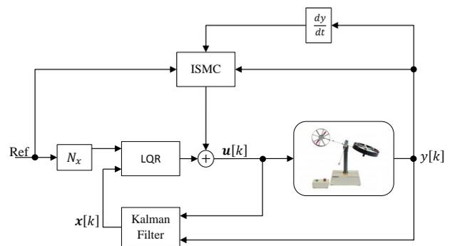
**Fig. 3:** The proposed system model with the LQG controller (LQR + Kalman filter) and the ISMC correction.
