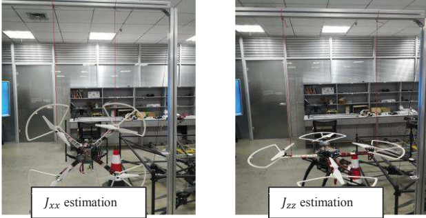
Fig. 4. Bifilar pendulum setup for estimating the moments of inertia.
