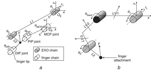
Fig. 2 Conceptual design of improved hand EXO device
