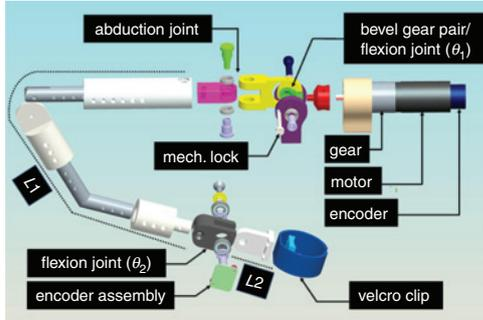
Fig. 5 CAD model of proposed finger mechanism (exploded view)
