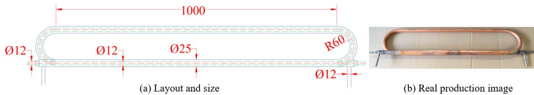
21 22 Fig. 3. The structure of the novel concentric tubes heat exchanger
