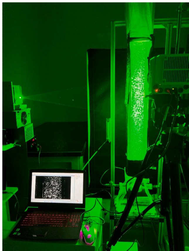
Fig. B1. Experimental set-up of the bubble column (Case 3).
