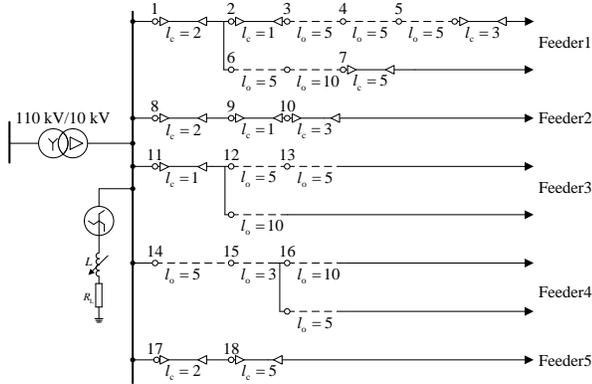
Fig. 5. 10 kV simulation model of RG distribution system.
