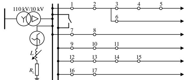
Fig. 13. Network structure of 10 kV substation.
