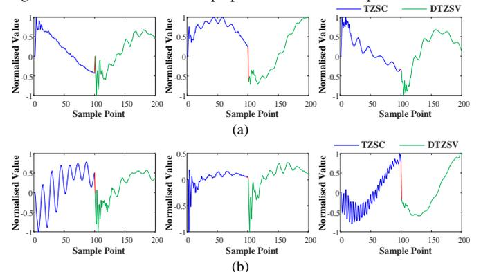
Fig. 7. Splicing waveforms of TZSC and DTZSV collected in (a) fault sections and (b) sound sections.
