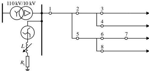
Fig. 11. Network structure of RTDS system.
