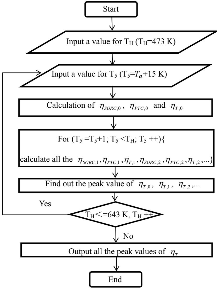
Fig. 14. Determination of peak solar thermal power efficiency with TH.
