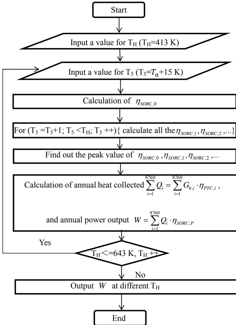
Fig. 19. Determination of maximum annual power output with  $T_H$ .
