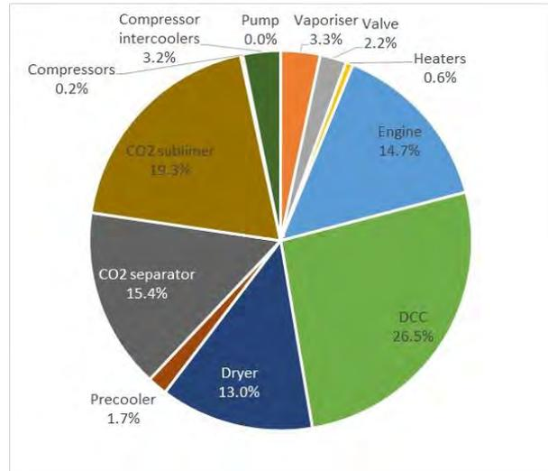
Figure 4: Percentage shares of exergy destruction based on the types of equipment in the cryogenic EGR case
