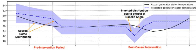
**Figure 1: Causal effects (non-obvious) of nacelle angle ( $X$ ) on generator stator temperature ( $y$ ) during anomaly in Yaw system using BSTS Approach (Statistically Insignificant). Probability of random occurrence  $p = 24.88\%$  and 95% interval of percentage change in  $X$  and  $y = [-3.44\%, 1.73\%]$ .**
