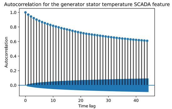
**Figure 2: Auto-correlation for the generator stator temperature time-series. The components are significantly non-zero, signifying non-random nature of the metric.**
