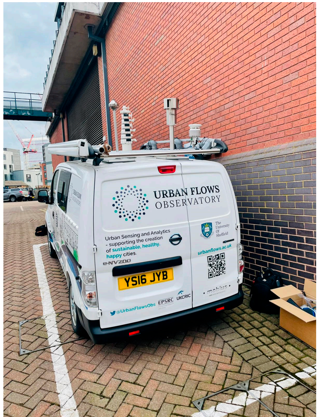
Figure 3. LCS-based AQ monitoring devices using RPi 3B+ at Urban Observatory, Sheffield Site.
