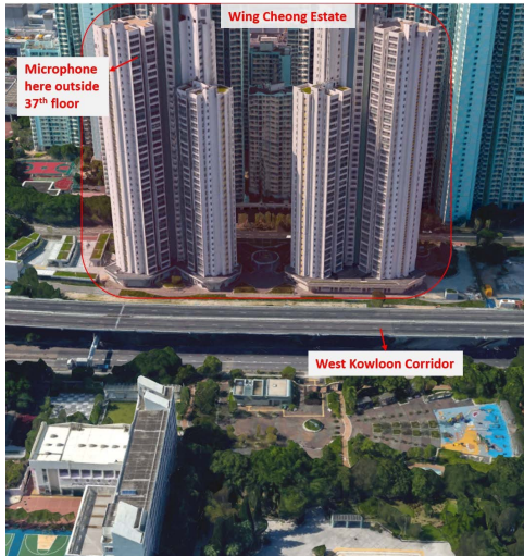
FIGURE 2. Google Earth's 3D-viewer snapshot, showing the measurement's physical environment and the microphone's exact 37th-floor location.
