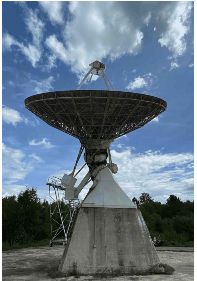
Figure 2. ARO 10 m telescope; photograph taken in 2020 September. The backplane and CHIME feed are visible at the telescope’s focus. The feed in the paraboloid focus is slightly offset toward the vertex.
