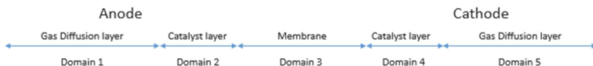
Figure 2. The geometry of the one-dimensional PEFC model.
