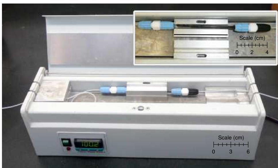
**Figure 42.** A photograph of the flow column, C2, within the chromatography column heater. Inset—A magnified view of the column *in-situ* with the top heating block removed.
