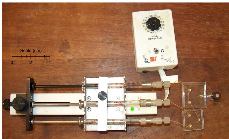
Figure 16. A photograph of a typical micro reactor set up.
