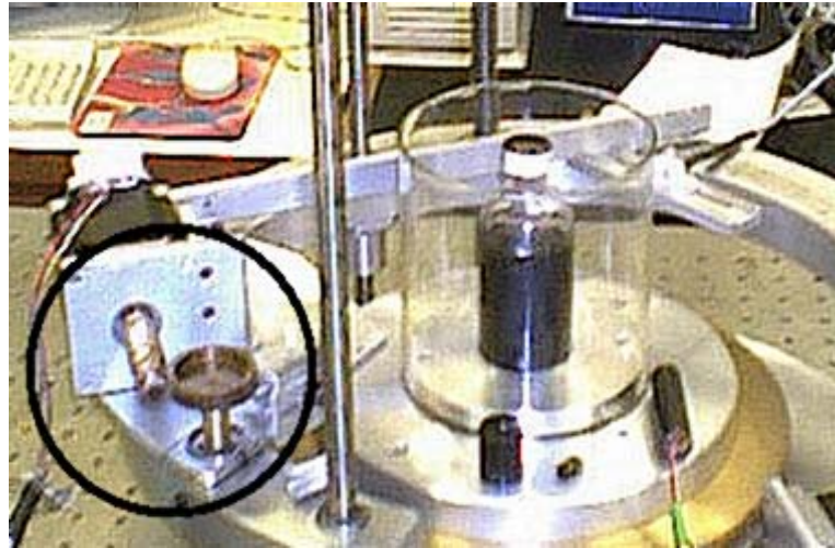
Figure [4-11] Photograph showing the stepper motor gears used to drive the laser beam fan arc required for gel scanning. The area circled shows the problematic fan beam scanning pivot and source of the scanning jitter.
