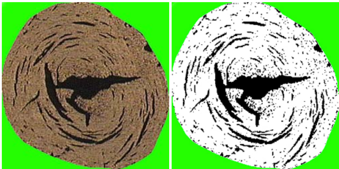
Figure 4.3.1 – Comparison of original Gilsocarbon particle image to threshold produced image. The green background was chosen because this colour does not occur naturally in graphite and therefore would not be picked up by any of the automatic selection tools incorporated into Adobe Photoshop CS.
