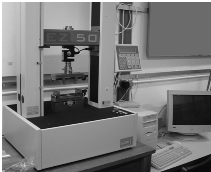
Figure 6.3.1 – Lloyd Instruments EZ50 universal testing machine with data acquisition PC.
