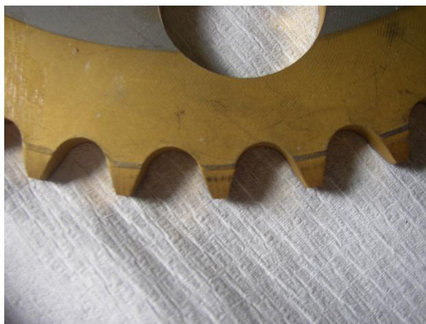
**Fig. 101** – Coated teeth after testing
