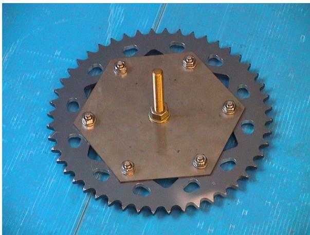
**Fig. 91** – Special sprocket holder utilized for RPS and PVD deposition process
