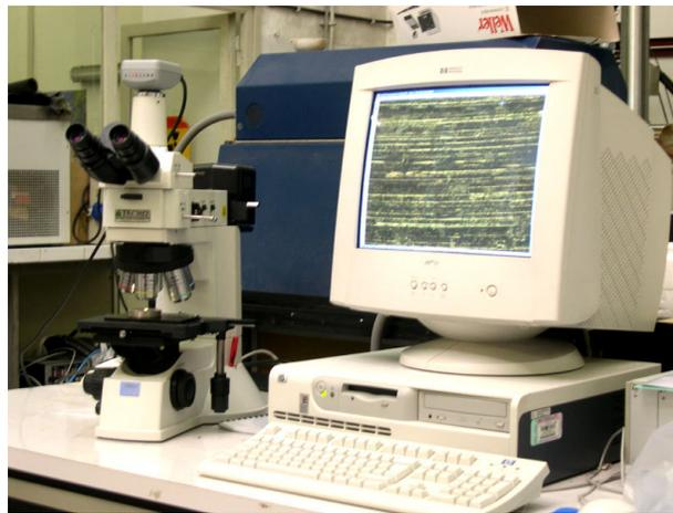
**Fig. 30** - Image analysis equipment: optical microscope + devoted software (Centro Sviluppo Materiali S.p.A.)
