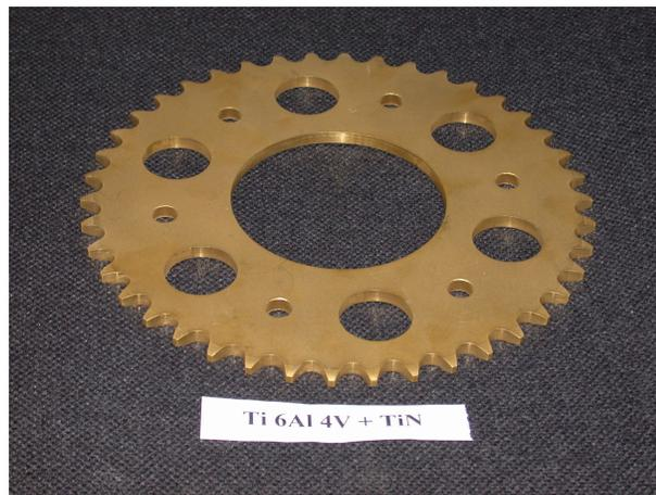
**Fig. 96**– Sprocket coated with the multilayer system, RPS Ti/TiN + PVD TiN
