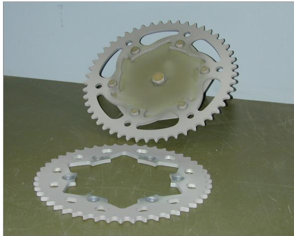
**Fig. 93** – Sprocket after RPS deposition
