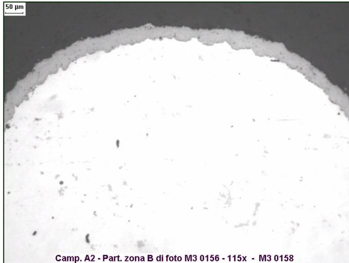
**Fig. 95** – Coating on a tooth section (plane of section parallel to the sprocket plane).
