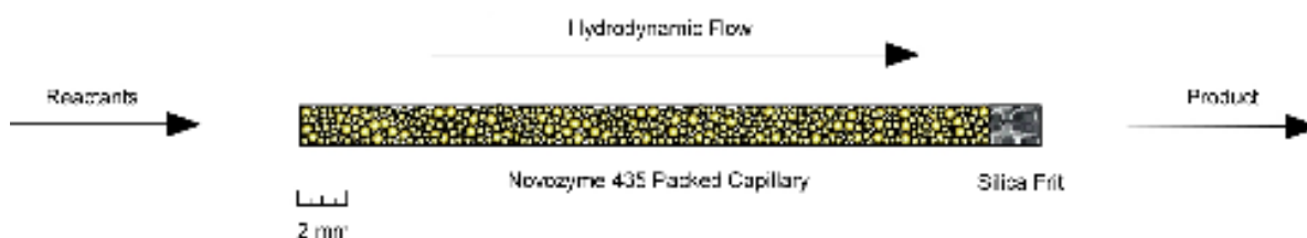
Figure 11: Set up of a miniaturised, packed bed, continuous flow reactor.
