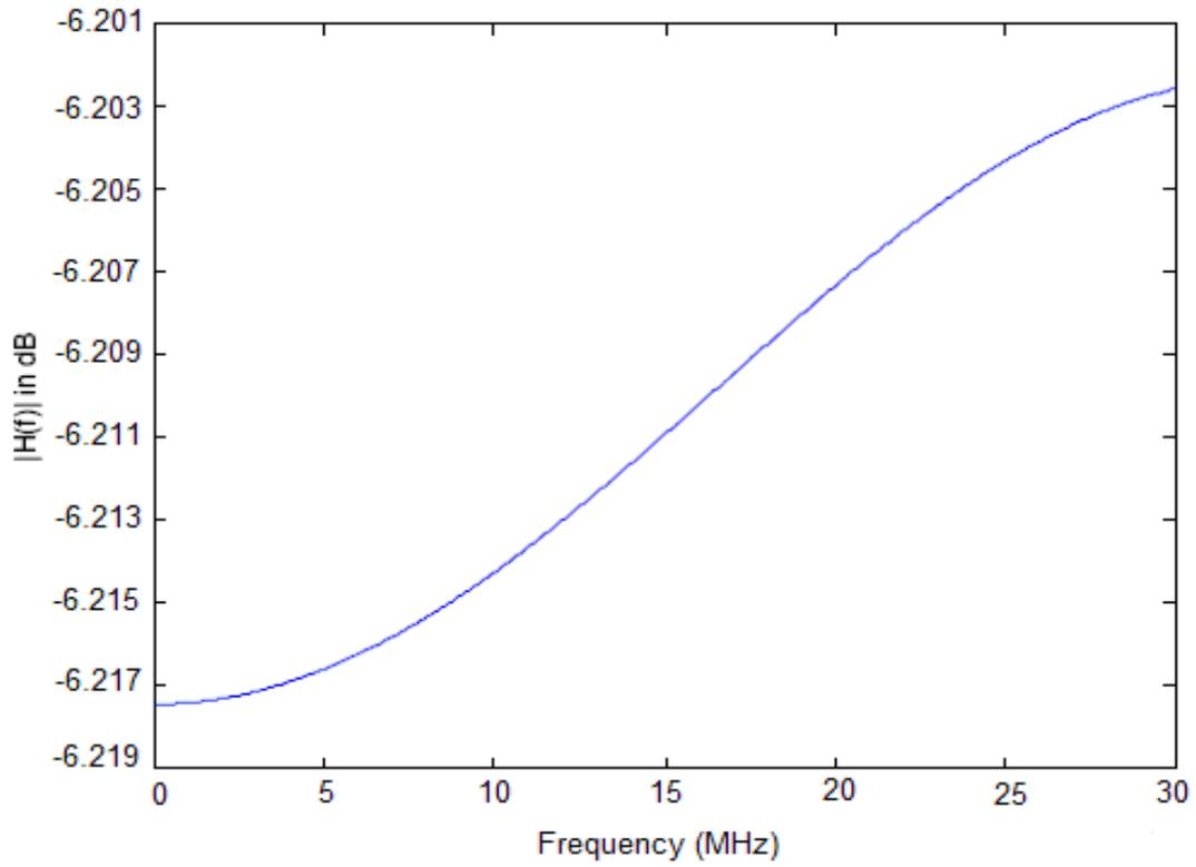
Figure 4.10 Plot of Power Line Model with  $Z_s = 50$  and  $Z_l = 70\Omega$  (cable length 1.5m)
