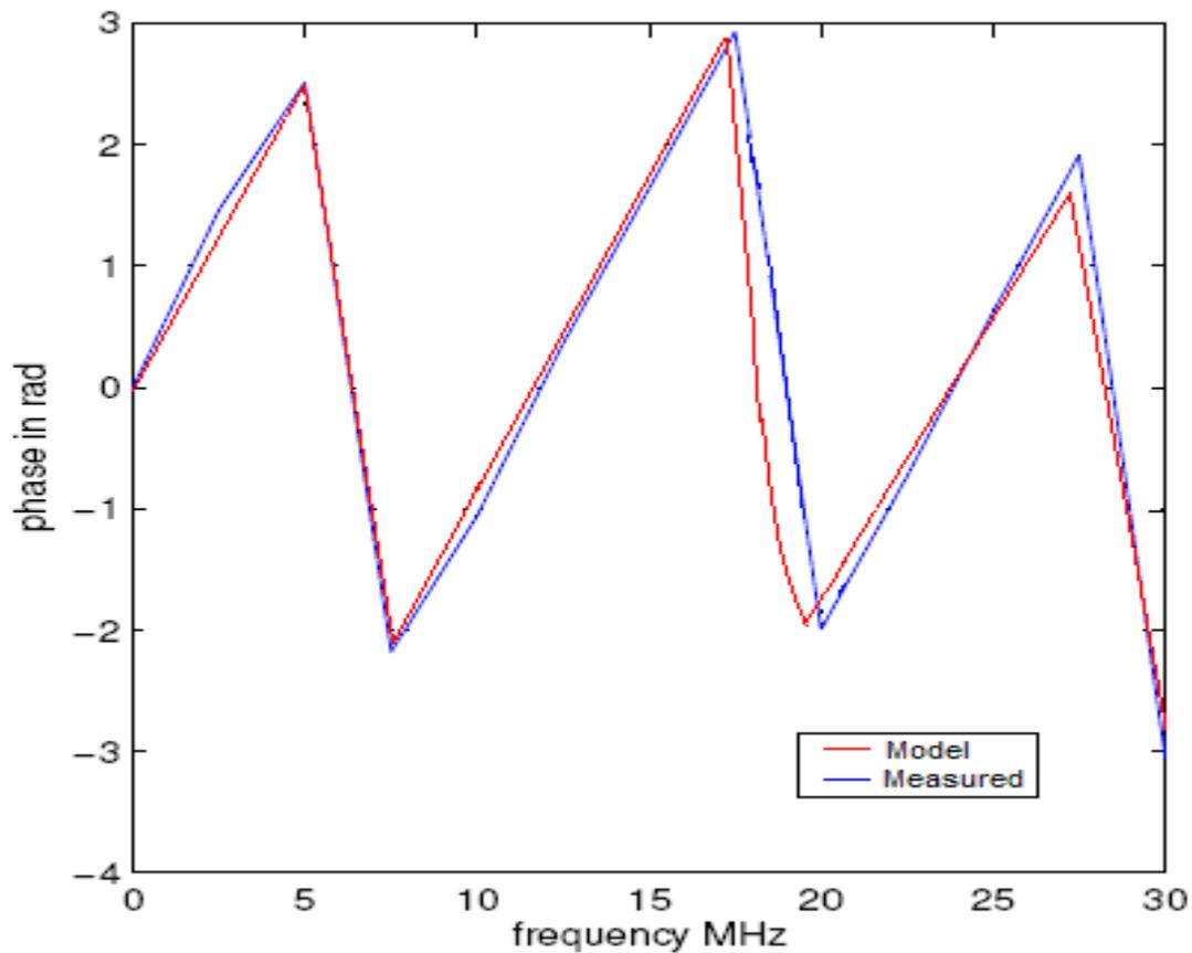
Figure 4.5 Phase spectrum of a 10m two core cable from 0 to 30MHz.
