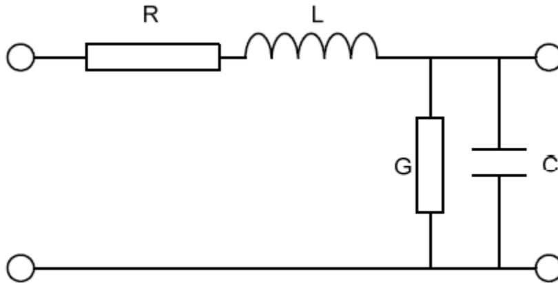
Figure 3.4 Lumped element transmission line model (figure abstracted from Minao and Maffucci, 2001).
