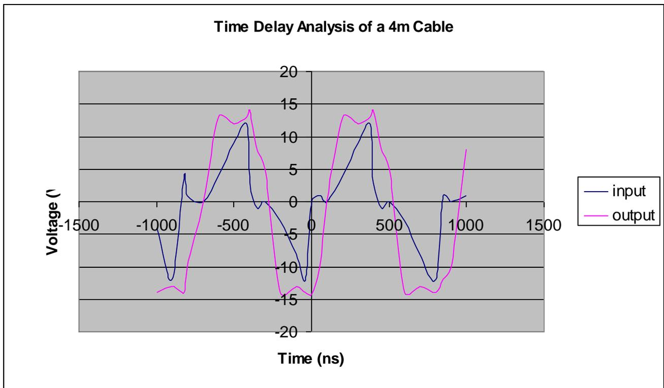
Figure 4.2 Input and output response of a 1MHz square wave signal.
