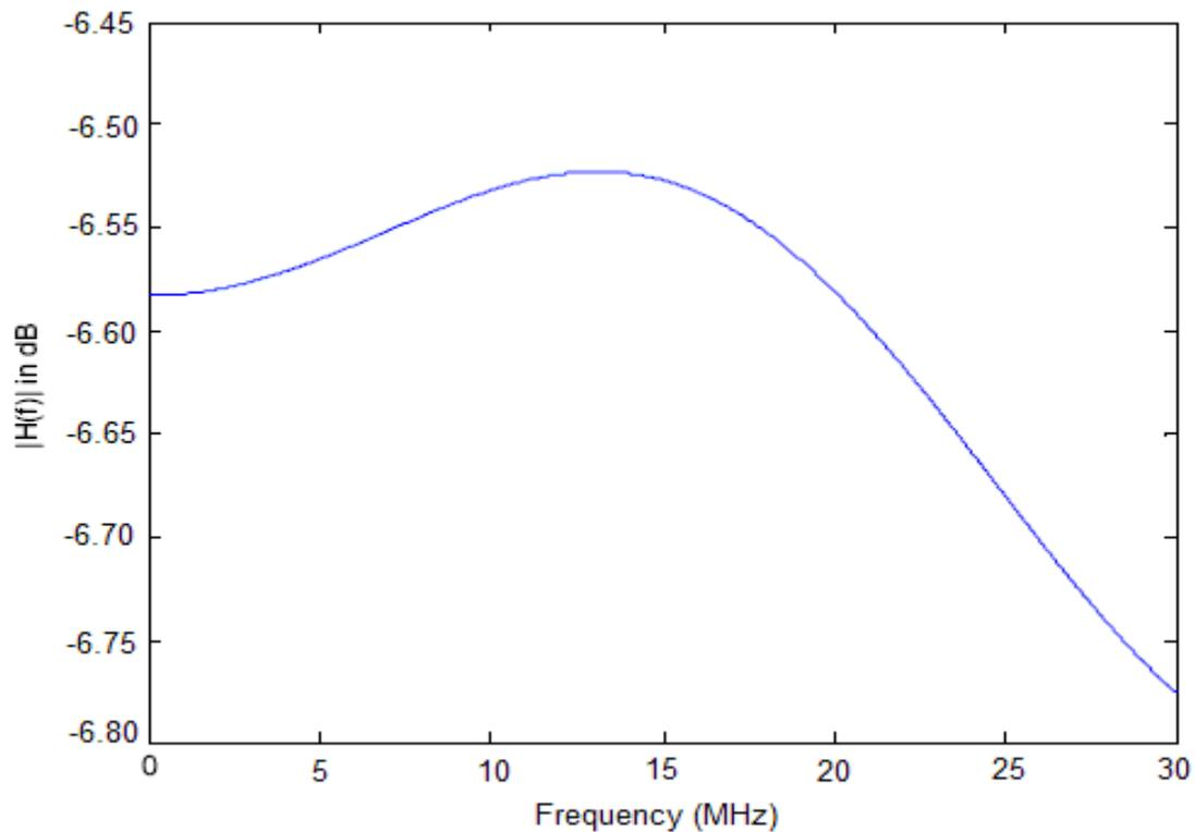
Figure 4.7 Plot of Power Line Model with  $Z_s = 50$  and  $Z_l = 60\Omega$  (cable length 3m)
