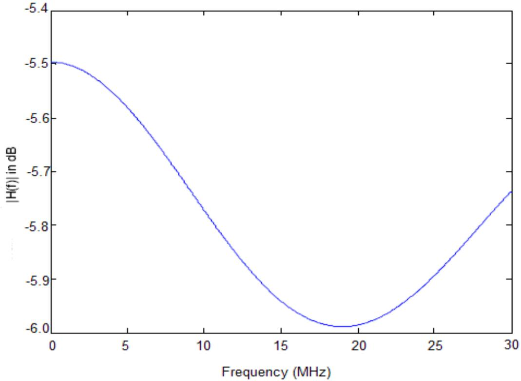
Figure 4.9 Plot of Power Line Model with  $Z_s = 60$  and  $Z_l = 100\Omega$  (cable length 3m)
