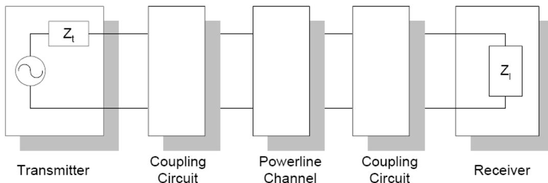
Fig. 2.9 A digital communications system for the power-line channel (figure abstracted from Dostert, 1997)
