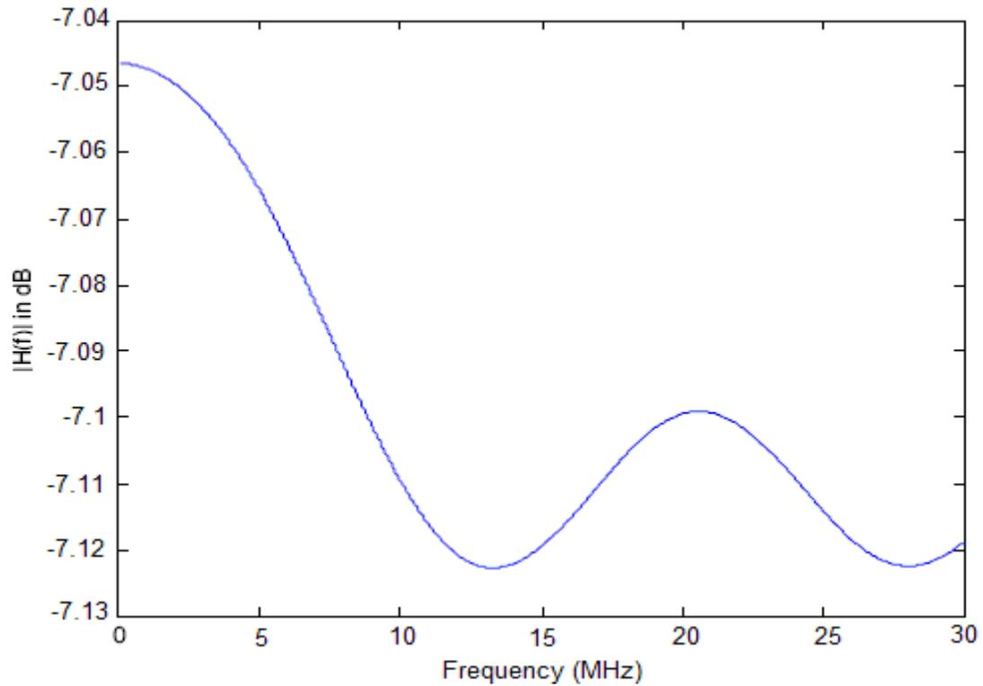
Figure 4.11 Plot of power line model with  $Z_s = 50$  and  $Z_l = 70$  (Cable length 6m)
