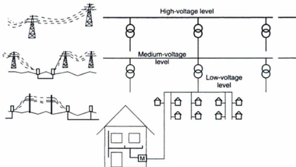
Fig 2.3 Structure of electrical supply networks (Figure abstracted from Hrasnica et al., 2004).
