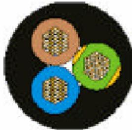
Figure 3.1 Cross Section of a Circular cord (figure abstracted from General cables, 2004).
