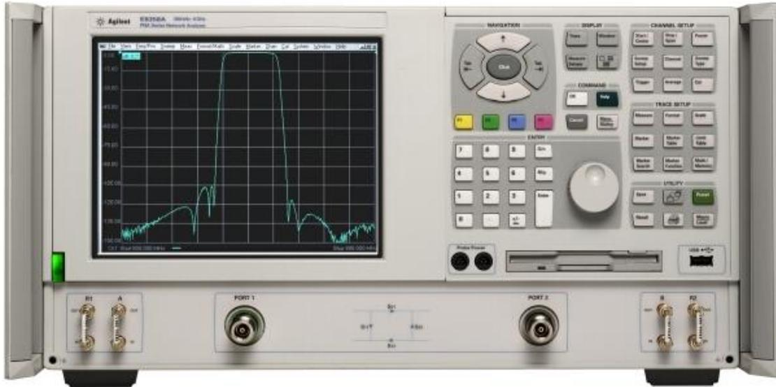
Figure 4.1 Agilent E8358A Network analyzer (figure abstracted from Agilent user guide, 2002).
