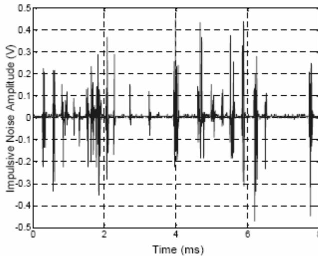
Figure 2.6 Asynchronous impulsive noise (in ms scale) [Figure abstracted from Liu et al., 2004].
