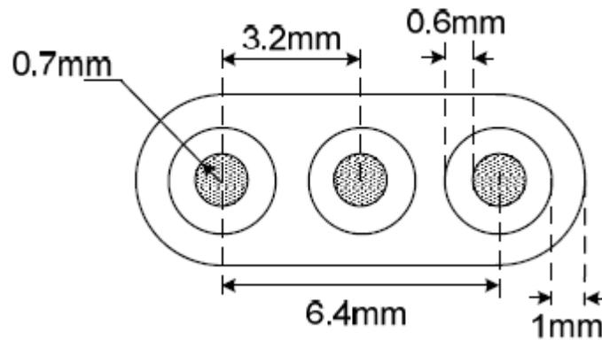
Figure 3.3 TPS Cable dimensions (figure abstracted from General cables, 2004)
