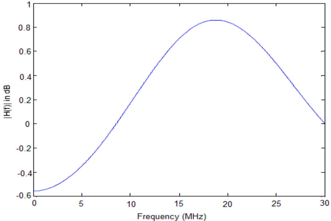
Figure 4.6 Plot of Power Line Model with  $Z_s = 10$  and  $Z_l = 60\Omega$  (cable length 3m)
