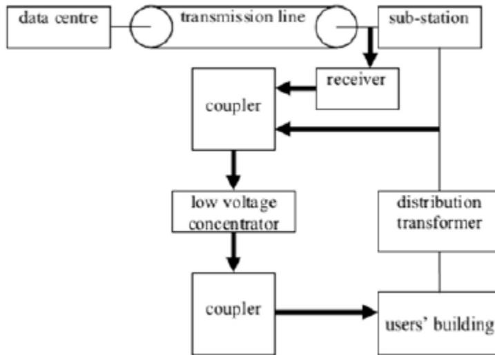
Fig.2.2 A simple PLC system (figure abstracted from Biswas, 2008).
