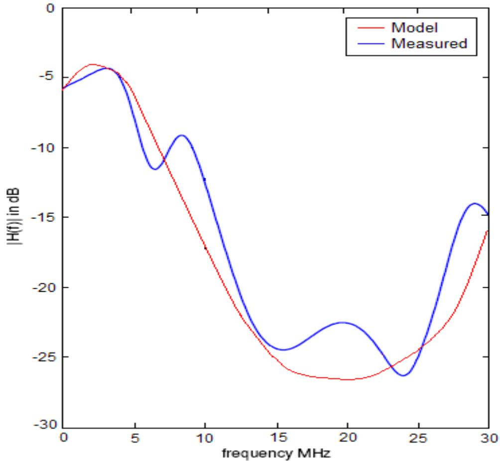
Figure 4.4 Attenuation of a 10m two core cable from 0 to 30MHz.
