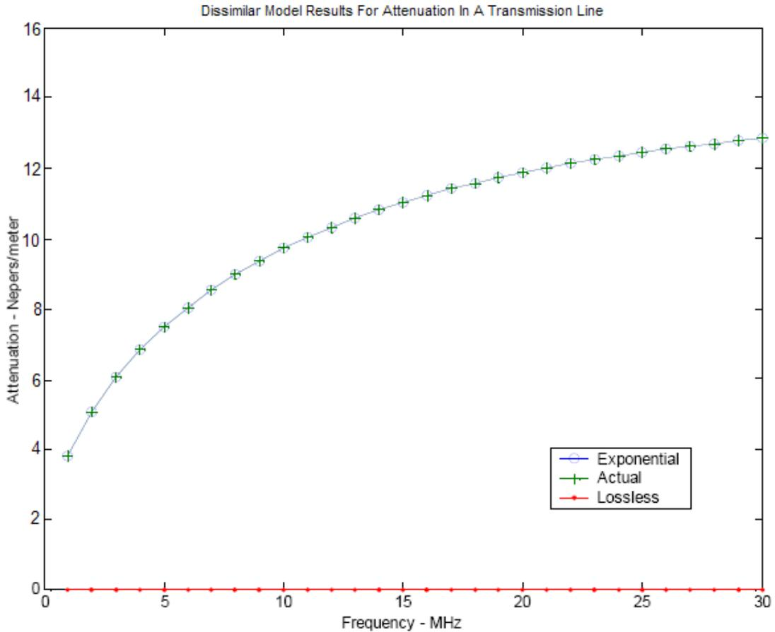
Figure 4.3 Attenuation results of different models from 1MHz to 30MHz.
