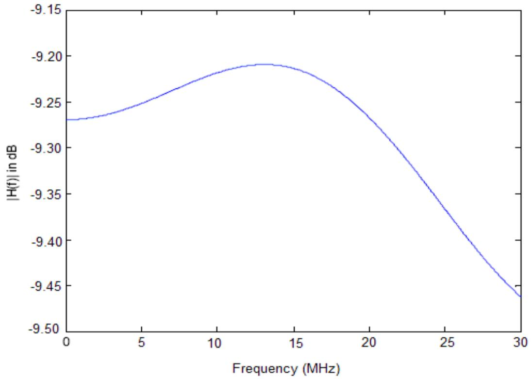
Figure 4.8 Plot of Power Line Model with  $Z_s = 60$  and  $Z_l = 60\Omega$  (cable length 3m)
