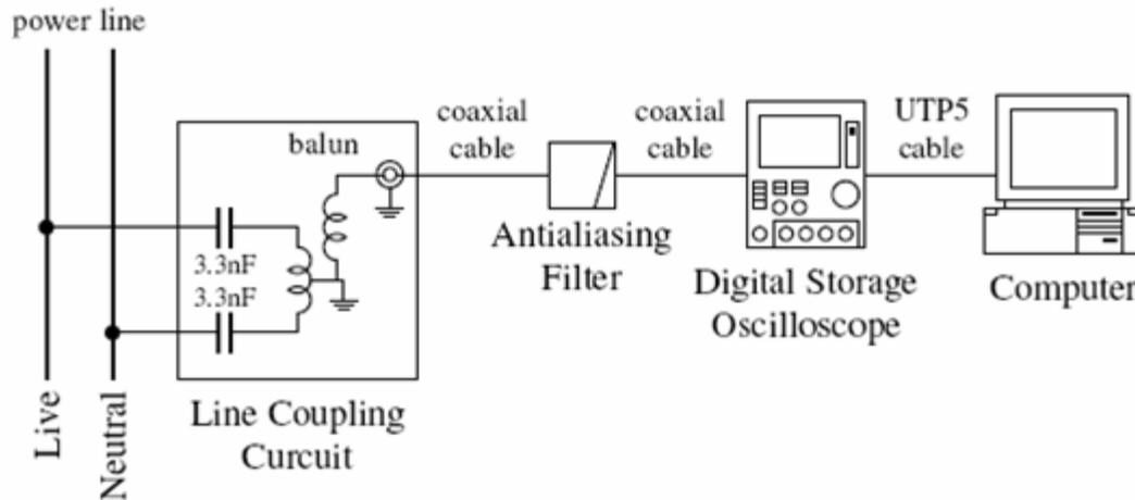
Fig. 2.8 System for measuring power line noise [Figure abstracted from Umehara et al., 2006].
