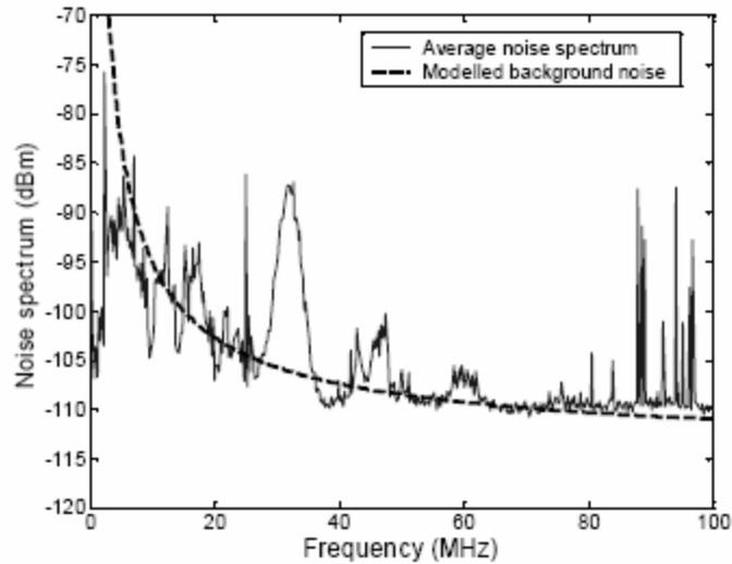
Figure 2.5 Background noise and its approximation [Figure abstracted from Liu et al., 2004].
