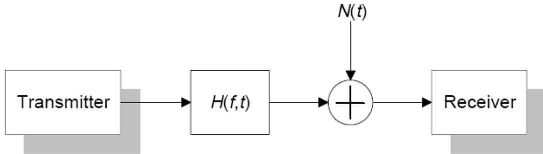
Figure 2.12 A simplified model of the power-line channel (Figure abstracted from Dostert, 1997)
