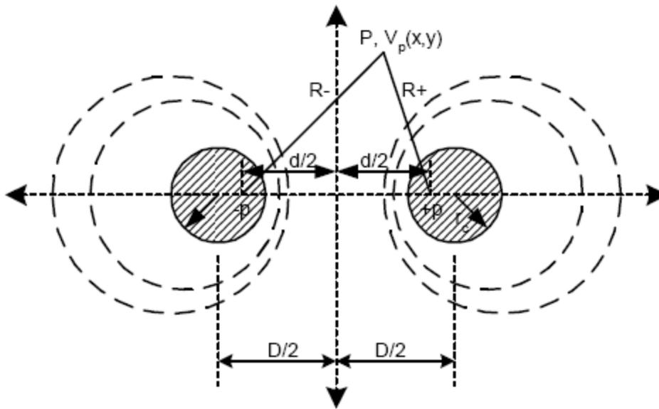
Figure 3.5 Cross sectional view of a two-wire transmission line (figure abstracted from Popovic, 1971).
