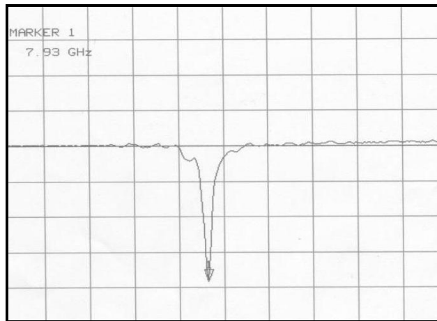
Figure 2.11: Graphical image from the Network Analyzer demonstrating the sharp peak obtained when the resonant frequency of the cavity has been achieved. In this example the optimum frequency is shown as 7.93 GHz.
