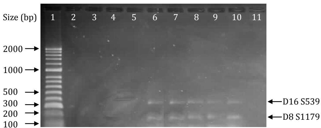
Figure 3.22: PCR amplification of DNA eluted from the microfluidic DNA extraction system using PCR reagents. UV transilluminator image of slab-gel electrophoresis results from DNA eluted in PCR reagents. Lane 1: DNA size ladder; Lanes 2-9: sequentially eluted DNA fractions; Lane 10: positive control and Lane 11: negative no DNA control.
